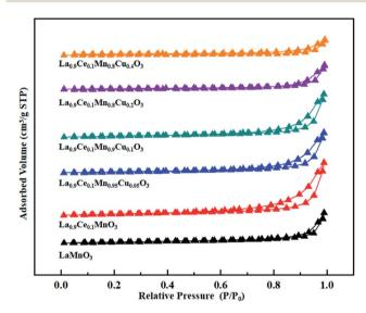
Fig. 3 N<sub>2</sub> adsorption-desorption isotherms of  $La_{1-x}Ce_xMn_{1-y}Cu_yO_3$  ( $x=0,\ 0.1,\ y=0,\ 0.05,\ 0.1,\ 0.2,\ 0.4$ ) catalysts.
