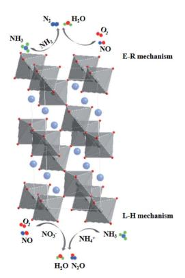
Fig. 9 Mechanism of  $NH_3\mbox{-}SCR$  Denitrification on Lanthanum–Manganese Perovskite Catalyst Surface at 200  $^{\circ}C.$
