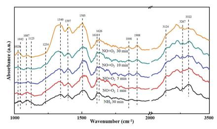
Fig. 7 DRIFT spectra of  $La_{0.9}Ce_{0.1}Mn_{0.8}Cu_{0.2}O_3$  exposed to NO at various temperatures. Reaction condition:  $[NH_3] = [NO] = 500$  ppm,  $[O_2] = 5\%$ , and  $N_2$  balance.
