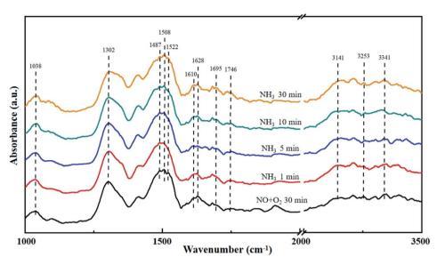
Fig. 8 DRIFT spectra of  $La_{0.9}Ce_{0.1}Mn_{0.8}Cu_{0.2}O_3$  exposed to  $NH_3$  at various temperatures. Reaction condition:  $[NH_3] = [NO] = 500$  ppm,  $[O_2] = 5\%$ , and  $N_2$  balance.
