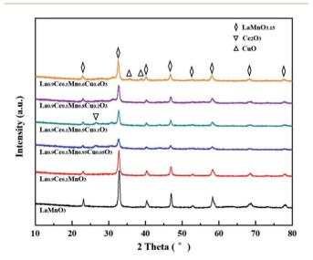
Fig. 1 XRD patterns of  $La_{1-x}Ce_xMn_{1-y}Cu_yO_3$  (x=0, 0.1, y=0, 0.05, 0.1, 0.2, 0.4) catalysts.
