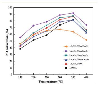
Fig. 6 NO conversion of the  $La_{1-x}Ce_xMn_{1-y}Cu_yO_3$  (x=0, 0.1, y=0, 0.05, 0.1, 0.2, 0.4) catalysts.
