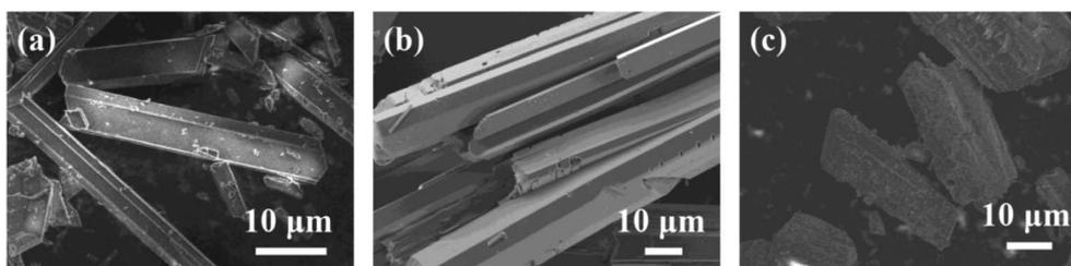
Fig. 8 SEM images of CaSO<sub>4</sub>: (a) without the scale inhibitor, (b) with 4 mg L<sup>-1</sup> PASP, and (c) with 4 mg L<sup>-1</sup> PASP-ED<sub>2</sub>A.
