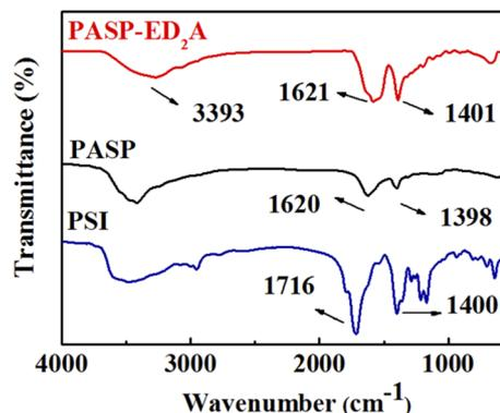
Fig. 3 FTIR spectra of PSI, PASP and PASP-ED<sub>2</sub>A.
