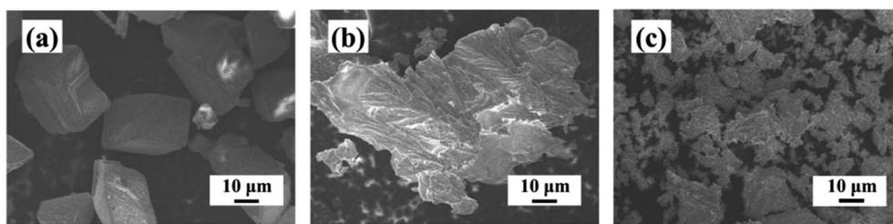
Fig. 7 SEM images of CaCO<sub>3</sub>: (a) without scale inhibitor, (b) with 30 mg L<sup>-1</sup> PASP, and (c) with 30 mg L<sup>-1</sup> PASP-ED<sub>2</sub>A.
