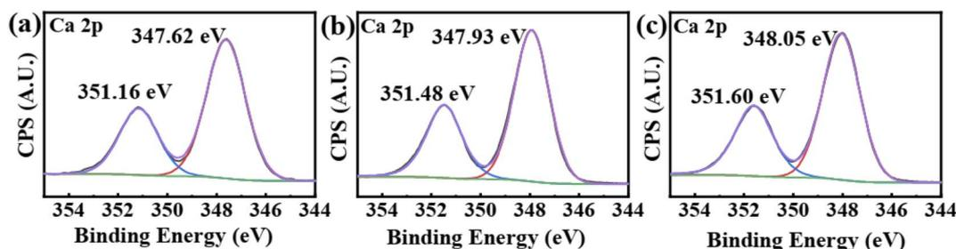
Fig. 11 XPS spectra of Ca 2p in CaSO<sub>4</sub> with different scale inhibitor. (a) Without antiscalant (b) with 4 mg L<sup>-1</sup> PASP (c) with 4 mg L<sup>-1</sup> PASP-ED<sub>2</sub>A.
