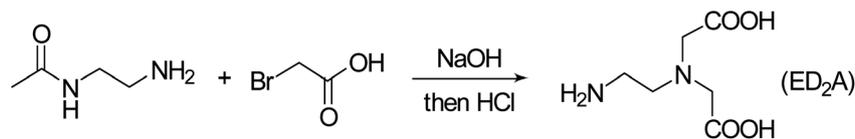
Fig. 1 Synthesis route of ED<sub>2</sub>A.
