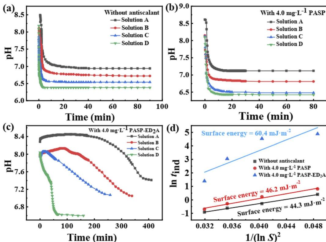
Fig. 12 pH–time curves of (a) blank CaCO<sub>3</sub> solution and the solutions with (b) 4.0 mg L<sup>-1</sup> PASP and (c) 4.0 mg L<sup>-1</sup> PASP–ED<sub>2</sub>A as well as (d) relation between ln  $t_{ind}$  and  $1/(\ln S)^2$  with or without the scale inhibitors.
