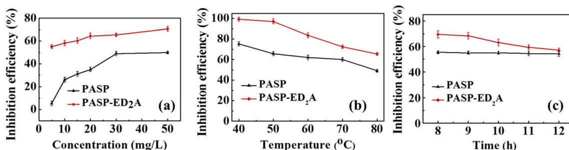
Fig. 5 Inhibition efficiency of PASP-ED<sub>2</sub>A and PASP towards  $\text{CaCO}_3$  scale versus (a) inhibitor concentration, (b) test temperature, and (c) test time.
