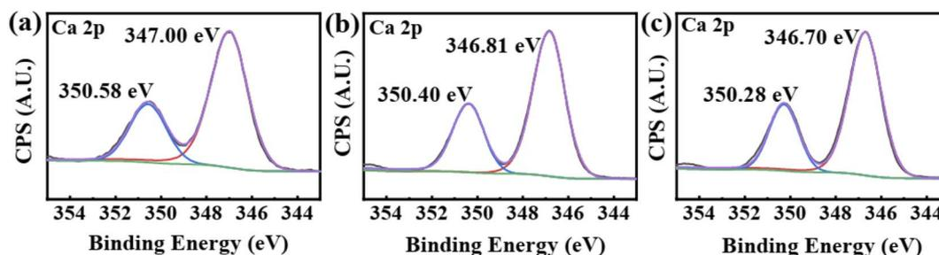
Fig. 10 XPS spectra of Ca 2p in CaCO<sub>3</sub> with different scale inhibitor. (a) Without antiscalant (b) with 30 mg L<sup>-1</sup> PASP (c) with 30 mg L<sup>-1</sup> PASP-ED<sub>2</sub>A.
