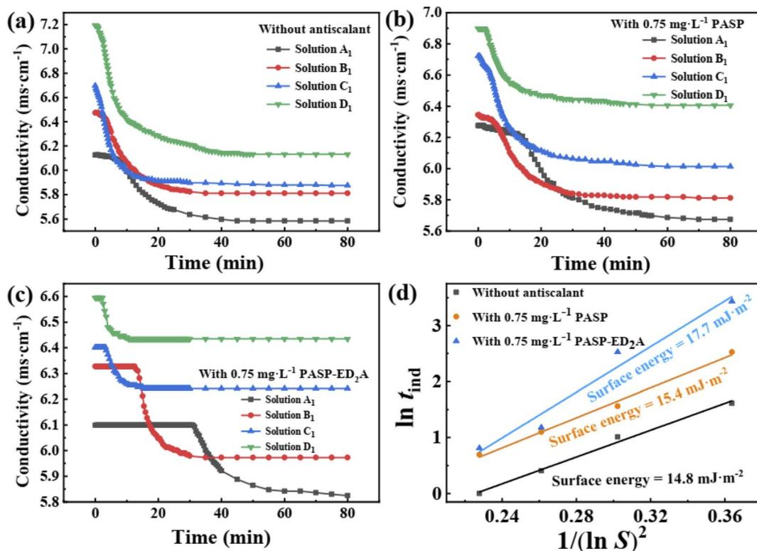
Fig. 13 Conductivity–time curves of CaSO<sub>4</sub> crystals formed without antiscalant (a), with 0.75 mg L<sup>-1</sup> PASP (b), and with 0.75 mg L<sup>-1</sup> PASP–ED<sub>2</sub>A (c), as well as relation between ln t<sub>ind</sub> and 1/(ln S)<sup>2</sup> with and without scale inhibitors (d).
