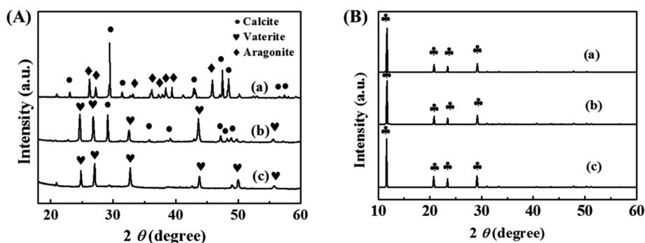
Fig. 9 XRD patterns of CaCO<sub>3</sub> scales formed in (A) aqueous solution of CaCO<sub>3</sub> ((a) without the scale inhibitor, (b) with 30 mg L<sup>-1</sup> PASP, and (c) with 30 mg L<sup>-1</sup> PASP-ED<sub>2</sub>A) and (B) aqueous solution of CaSO<sub>4</sub> ((a) without the scale inhibitor, (b) with 4 mg L<sup>-1</sup> PASP, and (c) with 4 mg L<sup>-1</sup> PASP-ED<sub>2</sub>A).
