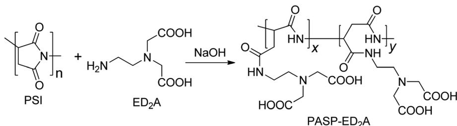
Fig. 2 Synthesis route of PASP-ED<sub>2</sub>A derivative.
