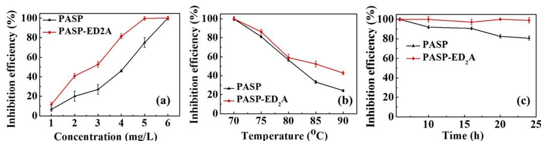
Fig. 6 Inhibition efficiency of PASP-ED<sub>2</sub>A and PASP towards  $\text{CaSO}_4$  scale versus (a) inhibitor concentration, (b) test temperature, and (c) test time.
