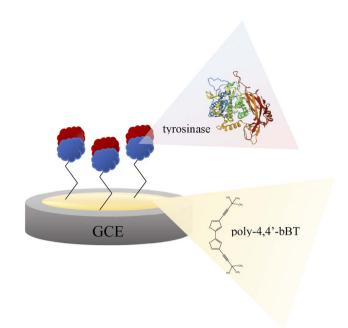
Fig. 2 Scheme of the bioplatform for epinephrine determination – glassy carbon electrode modified with poly-4,4′-bBT and tyrosinase.
