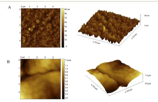
Fig. 3 (A) Representative AFM topography maps and surface 3D views of electrode surfaces modified with poly-4,4'-bis(2-methyl-3-butyn-2-ol)-2,2'-bithiophene and (B) poly-4,4'-bis(2-methyl-3-butyn-2-ol)-2,2'-bithiophene with tyrosinase;  $5 \times 5 \mu m$ .
