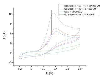
Fig. 5 Representative CV scans of the bare GC electrode (blue line), GCE modified with poly-4,4'-bBT (red line), and GCE/poly-4,4'-bBT/ Tyr (black line) in the presence of 200  $\mu$ M EP, and GCE/poly-4,4'-bBT/ Tyr (green line) in the absence of the analyte; applied potential range -0.2-0.8 V, scan rate 50 mV s $^{-1}$ , vs. Ag/AgCl.
