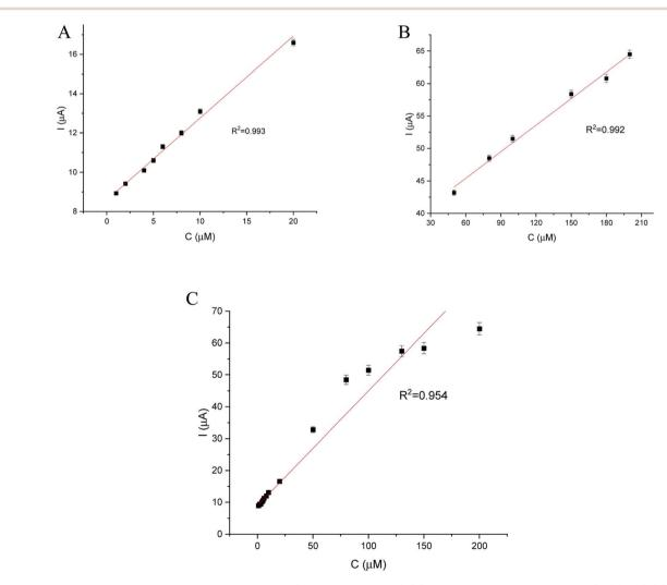
Fig. 7 Relationship between EP concentration and current (biosensor response): (A) – in a low concentration range (1–20  $\mu$ M), (B) – in a high concentration range (30–200  $\mu$ M), (C) – in a full concentration range (1–200  $\mu$ M).
