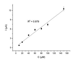
Fig. 9 Linear relationship of current and EP concentration (10–200  $\mu\text{M}).$
