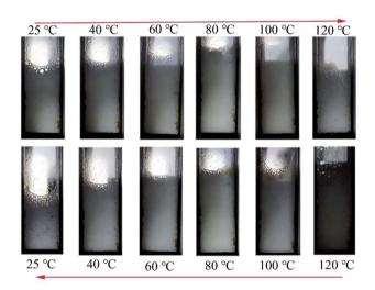
Fig. 7 Images of the foaming height of 0.2% GACB solution at a single heating procedure (from 25 to 120  $^{\circ}$ C) and cooling procedure (from 120  $^{\circ}$ C to 25  $^{\circ}$ C) at atmospheric pressure.
