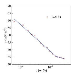
Fig. 3 Surface tension of the GACB solution as a function of concentration ( $T=25\,^{\circ}\text{C}$ ).
