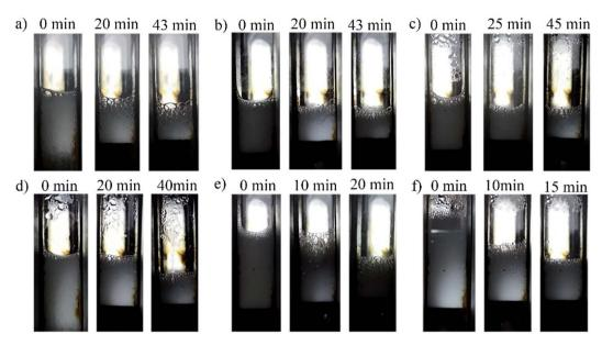
Fig. 6 Images of the GACB foam morphology under different temperatures: (a) 20 °C; (b) 40 °C; (c) 60 °C; (d) 80 °C; (e) 100 °C; (f) 120 °C.
