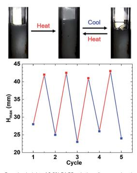
Fig. 8 Foaming height of 0.2% GACB solution after many heating (120  $^{\circ}\text{C})$  and cooling (25  $^{\circ}\text{C})$  procedures at atmospheric pressure.
