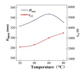
Fig. 4 Half-life period  $t_{1/2}$  and maximum foaming height  $H_{\rm max}$  of foams produced with 0.2% GACB solution at different temperatures.
