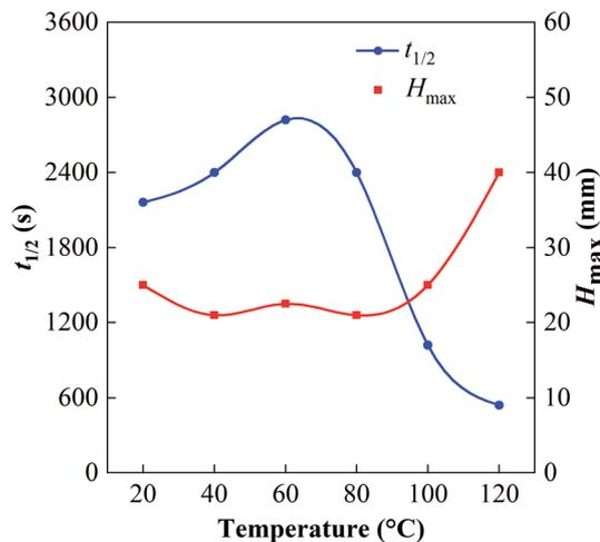
Fig. 5 The maximum height of the foam  $H_{\max}$  and the half-life period  $t_{1/2}$  of 0.2% GACB solution under different temperatures determined by the high-temperature and high-pressure visualization test.
