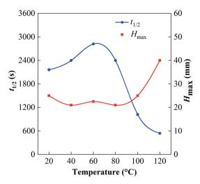
Fig. 5 The maximum height of the foam  $H_{\rm max}$  and the half-life period  $t_{1/2}$  of 0.2% GACB solution under different temperatures determined by the high-temperature and high-pressure visualization test.
