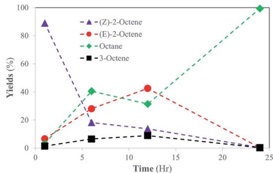
Fig. 5 Catalytic Conversion of Z-2-octene into isomerization and hydrogenation products at room temperature. The standard deviations of each data point are less than  $\pm 8\%$ . The large deviations in some data points are because some kinetics data points veered off from the overall results as outliers. This inconsistency was caused by running reactions independently from one another to preserve the PdNP : DSPC : Substrate ratio.
