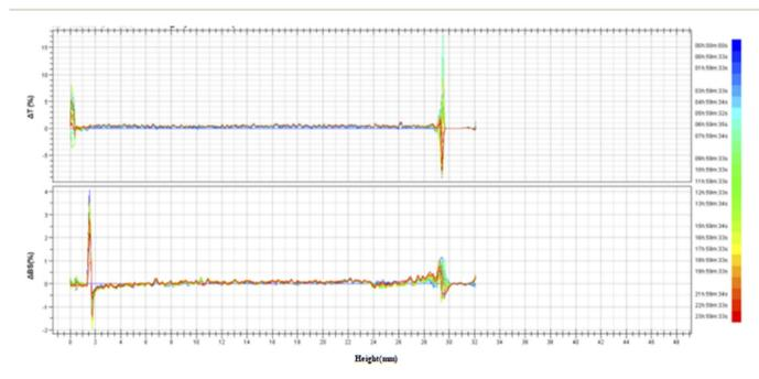
Fig. 6 Transmitted light/backscattered light reference spectrum of TG-KF. The stability of TG-KF was analyzed by multiple light scattering instrument according to the national standard methods (GB/T38431-2019). The multiple light scattering instrument uses near-infrared light as the light source, and has a transmitted light detector and a backscattered light detector.  $\Delta T$ : change value of transmitted light;  $\Delta BS$ : change value of backscattered light.
