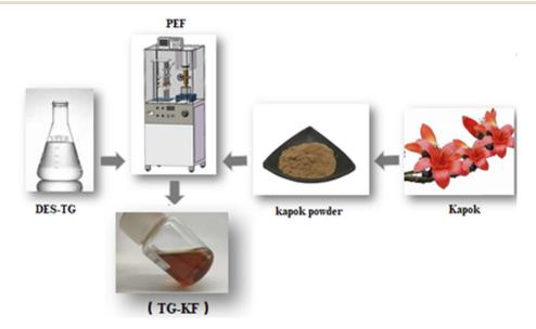
Fig. 3 Extraction process of TG-KF. Dried kapok were pulverized and mixed with 50% DES-TG in a ratio of 1:30, the mixture was extracted by using PEF equipment according to the instrument manual, the extracts were centrifuged and the supernatant were collected as TG-KF.
