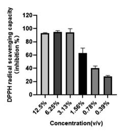
DPPH free radical scavenging rate of TG-KF. In vitro antioxidant capability of serial diluted TG-KF was tested by DPPH free radical scavenging assay. Data is expressed as mean SD, n = 3.
