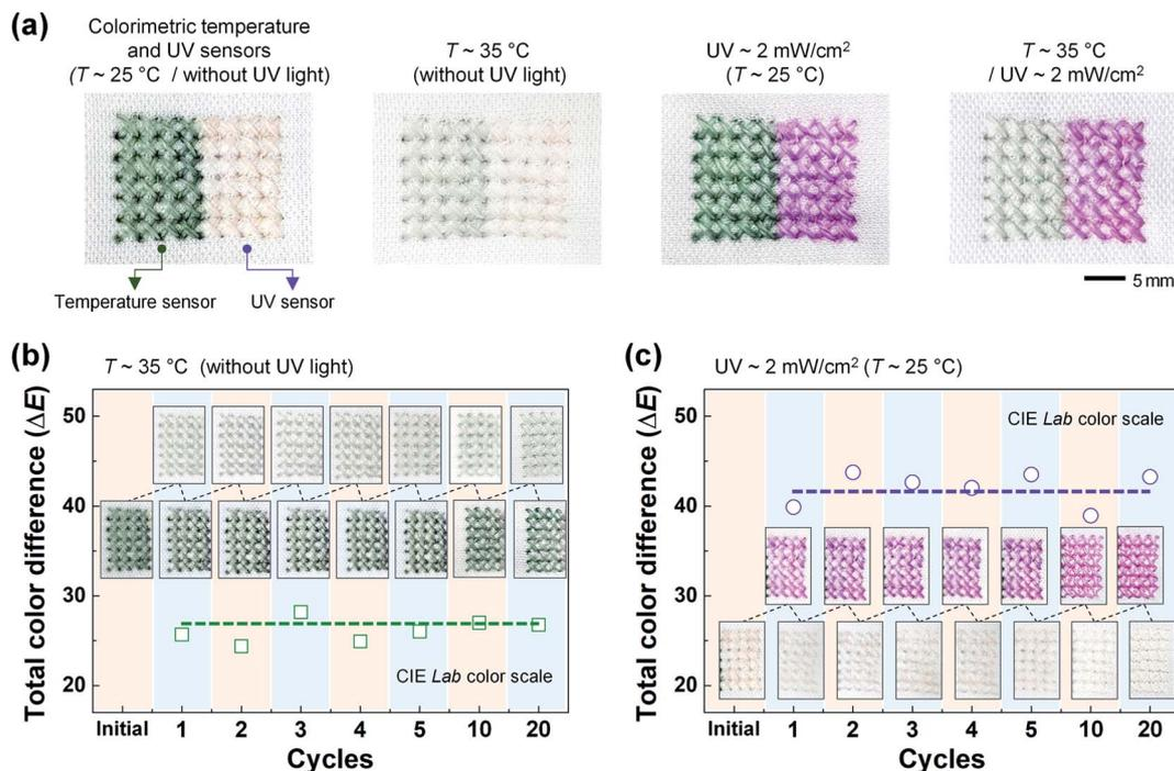
Fig. 5 (a) Textile-based colorimetric sensors woven from thermochromic and UV photochromic fibers repeatedly exposed to heat and/or UV light. (b) Color-change images and total color difference ( $\Delta E$ ) graph of the colorimetric temperature sensor. (c) Color-change images and  $\Delta E$  graph of the colorimetric UV sensor.
