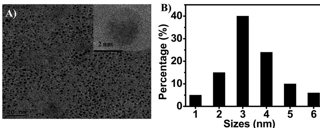
Fig. 1 (A) Typical TEM and HRTEM (inset) images of g-C<sub>3</sub>N<sub>5</sub>-dots. (B) Size distribution histograms of g-C<sub>3</sub>N<sub>5</sub>-dots.
