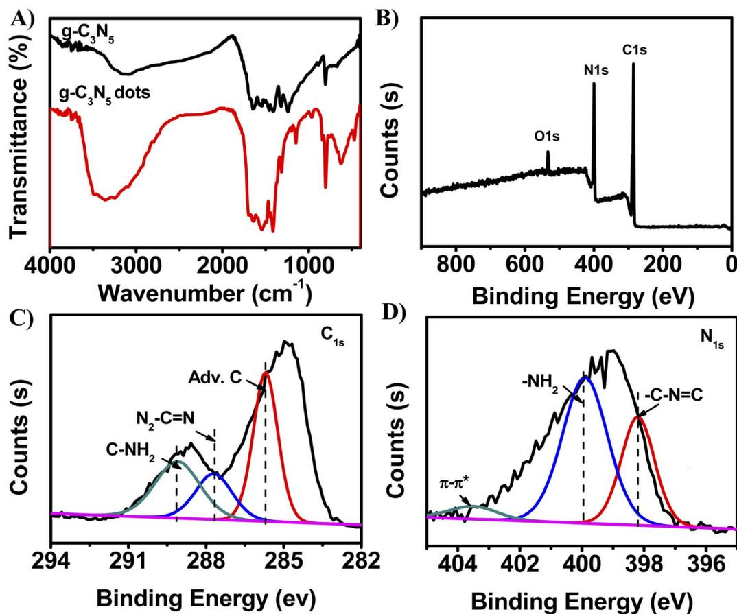
Fig. 2 (A) FT-IR spectra of g-C<sub>3</sub>N<sub>5</sub>-dots after hydrothermal treatment of 0.03 g g-C<sub>3</sub>N<sub>5</sub> powder with 0.3 g NaOH under 180 °C for 1 h. (B) XPS full spectra of g-C<sub>3</sub>N<sub>5</sub>-dots. High-resolution XPS of (C) C<sub>1s</sub> and (D) N<sub>1s</sub> of g-C<sub>3</sub>N<sub>5</sub>-dots prepared by hydrothermal treatment of 0.03 g g-C<sub>3</sub>N<sub>5</sub> powder with 0.3 g NaOH under 180 °C for 60 min.
