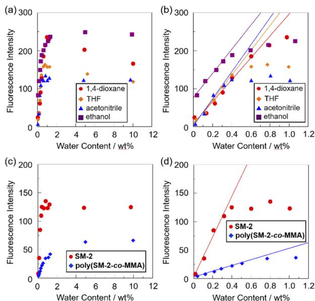
Fig. 5 Fluorescence peak intensity at around 420 nm of **SM-2** ( $\lambda^{\text{ex}} = 374$  or  $375$  nm) as a function of water content below (a) 10 wt% and (b) 1.1 wt% in 1,4-dioxane, THF, acetonitrile, and ethanol. Fluorescence peak intensity at around 420 nm of **SM-2** ( $\lambda^{\text{ex}} = 374$  nm) and **poly(SM-2-co-MMA)** ( $\lambda^{\text{ex}} = 375$  nm) as a function of water content below (c) 10 wt% and (d) 1.1 wt% in acetonitrile.
