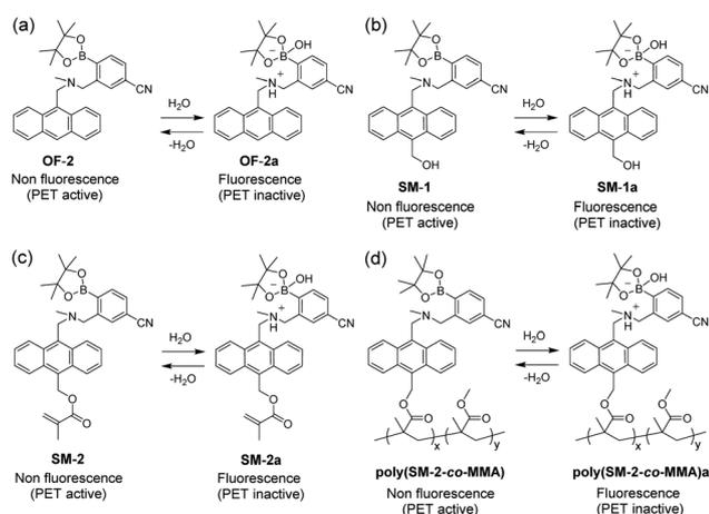
Fig. 1 Mechanisms of PET-type fluorescent sensors (a) **OF-2**, (b) **SM-1** (previous work), (c) **SM-2**, and (d) **poly(SM-2-co-MMA)** (this work) for detection of water in organic solvents and films.
