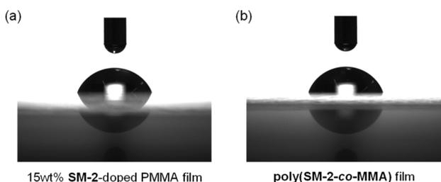
Fig. 10 (a) Water contact angle images of (a) 15 wt% SM-2-doped PMMA film and (b) poly(SM-2-co-MMA) film.
