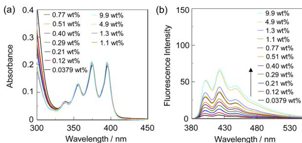
Fig. 6 (a) Photoabsorption and (b) fluorescence spectra ( $\lambda^{\text{ex}} = 375 \text{ nm}$ ) of poly(SM-2-co-MMA) in acetonitrile containing water (0.0379–9.9 wt%). The concentration of the solutions was adjusted so that the absorbance at 375 nm was ca. 0.2, that is, the concentration of SM-2 unit in poly(SM-2-co-MMA) was ca.  $2.0 \times 10^{-5} \text{ M}$ , which was the same as the case of SM-2 in Fig. 2.
