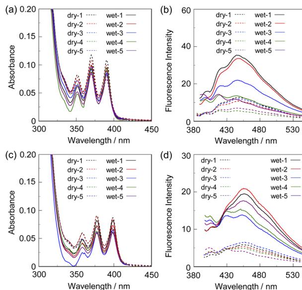
Fig. 8 (a) Photoabsorption and (b) fluorescence spectra ( $\lambda^{\text{ex}} = 368$  nm) of 50 wt% OF-2-doped PMMA film before (in dry process) and after (in wet process) exposure to moisture. (c) Photoabsorption and (d) fluorescence spectra ( $\lambda^{\text{ex}} = 377$  nm) of 50 wt% SM-2-doped PMMA film before (in dry process) and after (in wet process) exposure to moisture. For all the photoabsorption spectra, baseline-correction was made to be the same absorbance at 420 nm.
