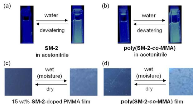
**Fig. 3** Photographs (under 365 nm irradiation) of acetonitrile solutions of (a) **SM-2** and (b) **poly(SM-2-co-MMA)** before and after addition of water and (c) 15 wt% **SM-2**-doped PMMA film and (d) **poly(SM-2-co-MMA)** film before and after exposure to moisture.
