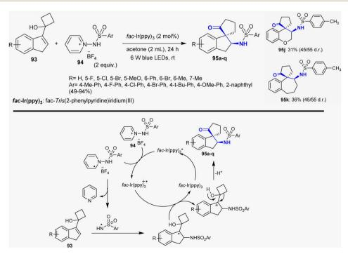
Scheme 33 Synthesis of β-aminoketones with the spiro-cyclic core.
