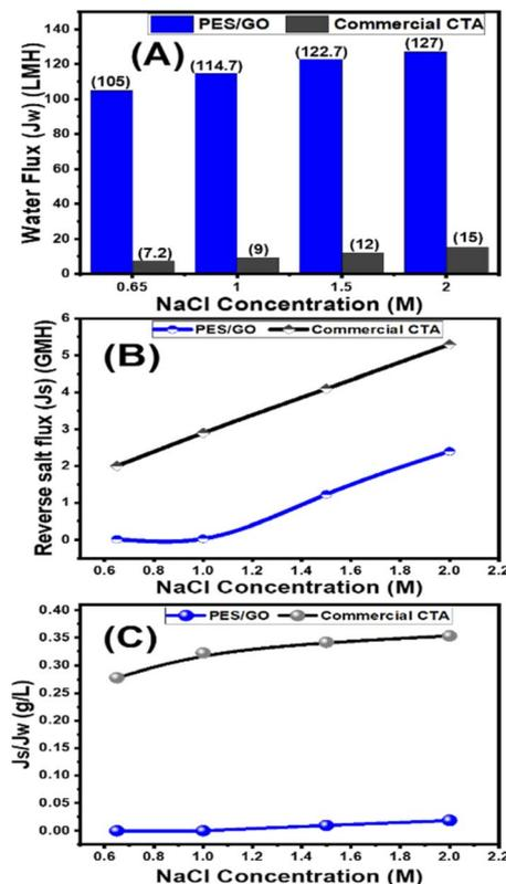
Fig. 8 Comparison of the (A) water flux ( $J_w$ ), (B) reverse salt flux ( $J_s$ ), and (C)  $J_w/J_s$  of the prepared PES/GO MMW FO membrane (SG3) with the woven commercial cellulose triacetate (CTA) membrane as a function of the NaCl concentration. Measurements were carried out at the same conditions.
