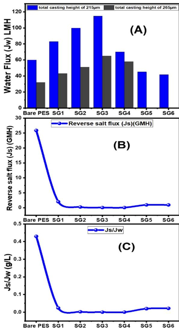
Fig. 6 PES/GO MMW FO membranes performance indicators; variation of (A) the water flux ( $J_w$ ) for the prepared membranes using 215  $\mu\text{m}$  and 265  $\mu\text{m}$  total casting thicknesses; (B) the minimum reverse salt flux ( $J_s$ ) and (C)  $J_w/J_s$  for the prepared membranes using 215  $\mu\text{m}$  total casting thickness versus the GO NSs wt%.
