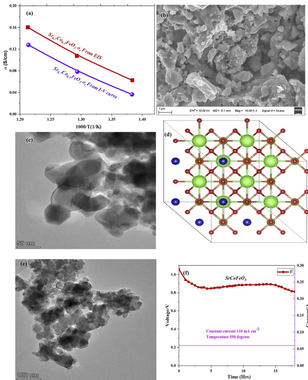
Fig. 7 (a) The total and ionic conductivity of synthesized electrolyte  $\text{Sr}_{0.7}\text{Co}_{0.3}\text{FeO}_3$  at different temperatures 550–450 °C, (b, c, e) SEM and HR-TEM morphology of  $\text{Sr}_{0.7}\text{Co}_{0.3}\text{FeO}_3$  while (d) the side view of the crystal structure of  $\text{Sr}_{0.7}\text{Co}_{0.3}\text{FeO}_3$  with 101 planes, (f) durability of  $\text{Sr}_{0.7}\text{Co}_{0.3}\text{FeO}_3$  at 550 °C.
