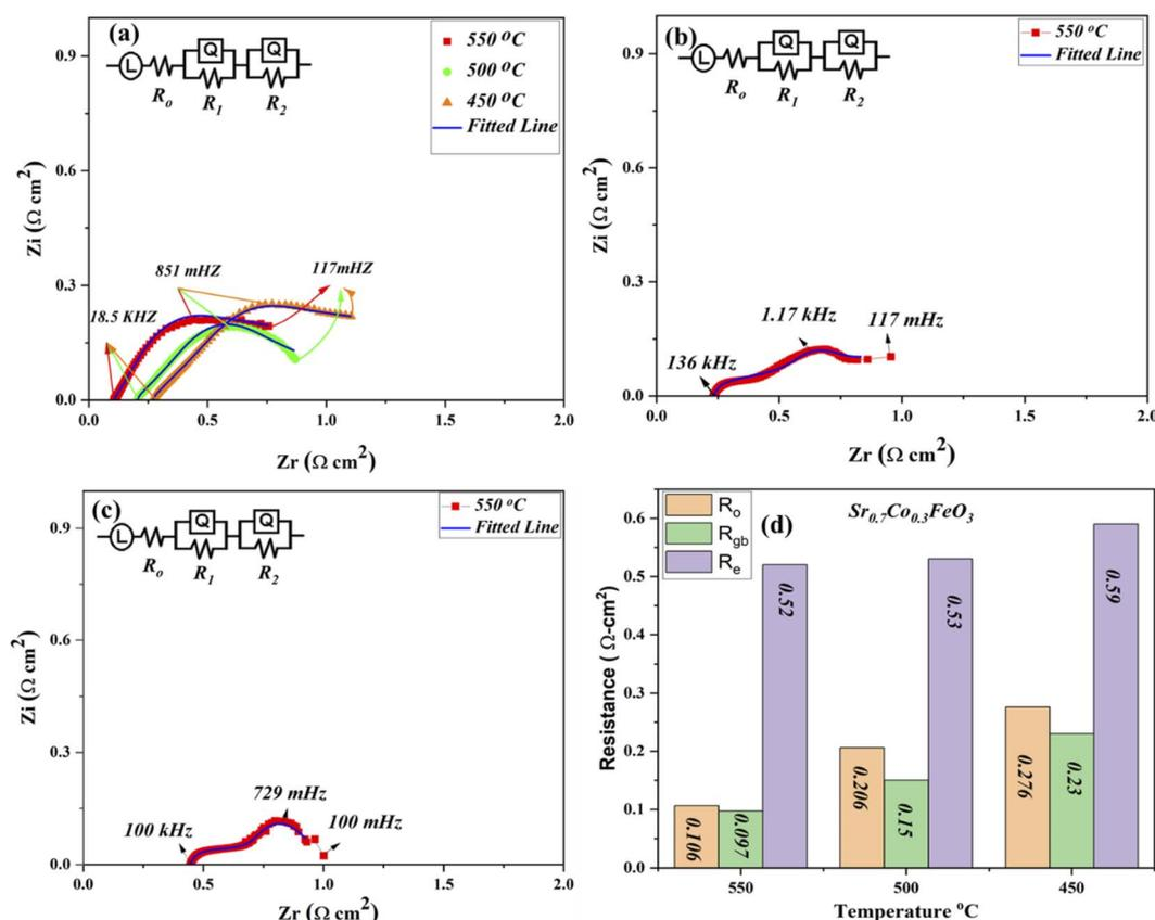
Fig. 4 (a) EIS spectra of Sr<sub>0.7</sub>Co<sub>0.3</sub>FeO<sub>3</sub> under H<sub>2</sub>/air at 550–450 °C, (b and c) EIS spectra of other compositions Sr<sub>0.7</sub>Co<sub>0.5</sub>FeO<sub>3</sub> and Sr<sub>0.7</sub>Co<sub>0.7</sub>FeO<sub>3</sub> under H<sub>2</sub>/air at 550 °C (d) comparison of EIS resistance values of Sr<sub>0.7</sub>Co<sub>0.3</sub>FeO<sub>3</sub> at 550–450 °C.
