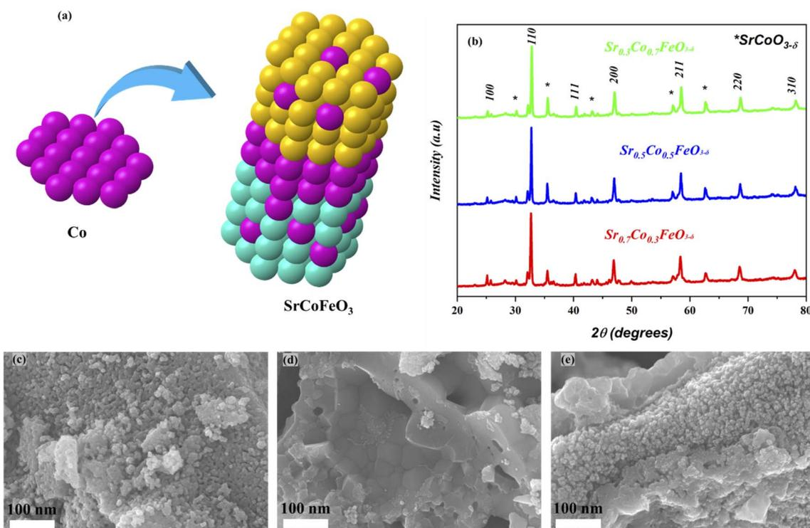
Fig. 1 (a and b) Crystal structure and XRD result of synthesized lattice  $\text{Sr}_{1-x}\text{Co}_x\text{FeO}_{3-\delta}$  sintered at 800 °C while (c–e) the FE-SEM images of  $\text{Sr}_{1-x}\text{Co}_x\text{FeO}_{3-\delta}$  ( $x = 0.3-0.7$ ) respectively.
