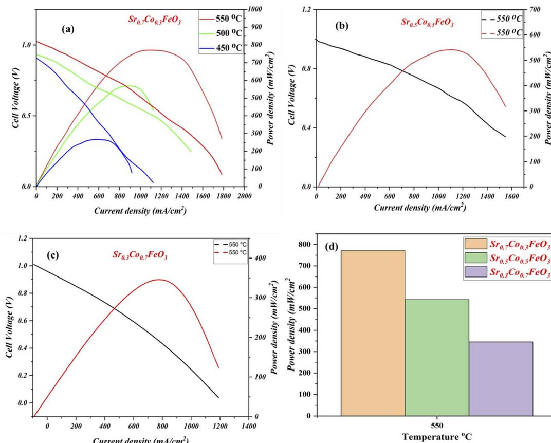
Fig. 5 (a–c) Fuel cell performance of  $\text{Sr}_{0.7}\text{Co}_{0.3}\text{FeO}_3$  under  $\text{H}_2/\text{air}$  at 550–450 °C, (d) comparison of Fuel cell performance of  $\text{Sr}_{1-x}\text{Co}_x\text{FeO}_3$  ( $x = 0.3–0.7$ ) at 550 °C.
