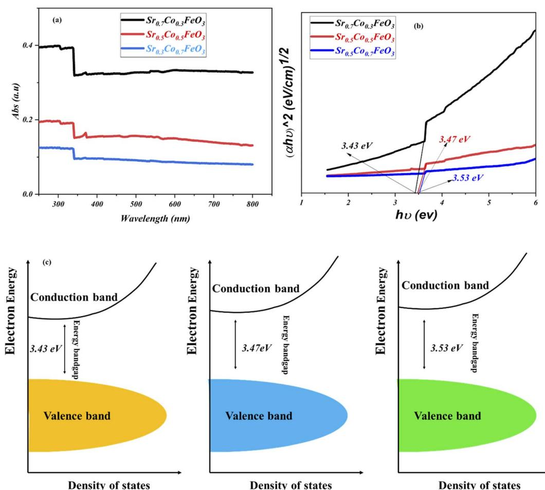
Fig. 6 (a and b) UV-visible spectra of  $\text{Sr}_{1-x}\text{Co}_x\text{FeO}_3$  ( $x = 0.3\text{--}0.7$ ), (c) energy bandgap diagram of all composition of comparison of  $\text{Sr}_{1-x}\text{Co}_x\text{FeO}_3$  ( $x = 0.3\text{--}0.7$ ).
