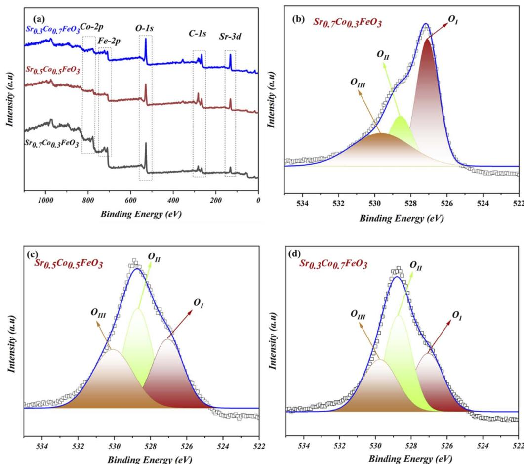
Fig. 2 (a) Full XPS (X-ray photoelectron spectroscopy) spectra of prepared SrCoFeO<sub>3</sub>, (b–d) O-1s spectra of Sr<sub>1-x</sub>Co<sub>x</sub>FeO<sub>3</sub> ( $x = 0.3-0.7$ ).
