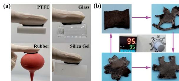
Fig. 4 (a) Digital photos of the hydrogel adhered to the surface of different substrates. (b) Re-modelling the hydrogel into different morphologies after dissolved into aqueous solution at  $95^\circ\text{C}$ .
