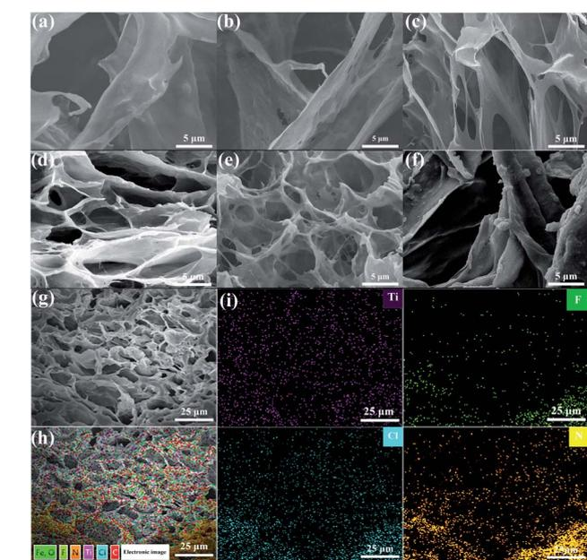
Fig. 1 SEM images of PVA/QCS-C/MXene hydrogels with different QCS-C contents. (a) PVA/QCS-C<sub>5</sub>/MXene, (b) PVA/QCS-C<sub>10</sub>/MXene, (c) PVA/QCS-C<sub>15</sub>/MXene, (d) PVA/QCS-C<sub>20</sub>/MXene, (e) PVA/QCS-C<sub>25</sub>/MXene, (f) PVA/QCS-C<sub>30</sub>/MXene, (g) SEM image of PVA/QCS-C<sub>15</sub>/MXene after  $\text{FeCl}_3$  cross-linking, (h) and (i) EDS images of (g).
