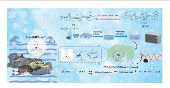
**Scheme 1** Schematic illustration of the preparation of PVA/QCS-C/MXene hydrogels for strain sensors.
