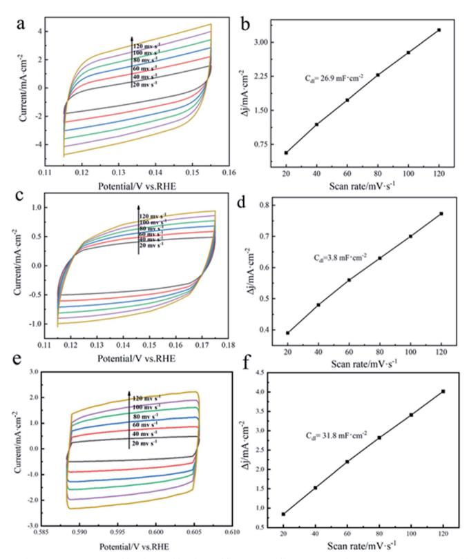
Fig. 6 Cyclic voltammetry curves of (a) TiVCT<sub>x</sub>@NF, (c) TiVCT<sub>x</sub> and (e) commercial Pt/C recorded from -6 to 94 mV vs. RHE at scan rates of 20, 40, 60, 80, 100 and 120 mV s<sup>-1</sup>. Estimated double-layer capacitances ( $C_{\rm cl}$ ) of (b) TiVCT<sub>x</sub>@NF, (d) TiVCT<sub>x</sub> and (f) commercial Pt/C.
