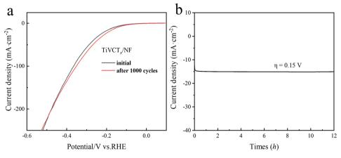
Fig. 9 (a) Polarization curves of  $TiVCT_x@NF$  initially and after 1000 CV cycles. (b) Current density *versus* time for  $TiVCT_x@NF$  at a 150 mV potential.
