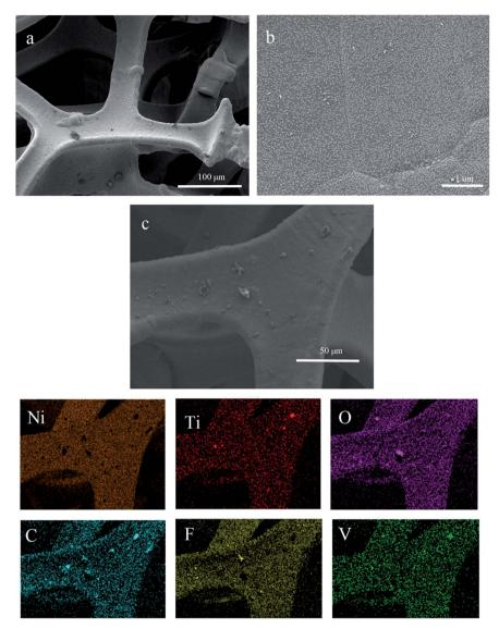
(a and b) SEM images of TiVCT<sub>x</sub>@NF. (c) Elemental mapping images of TiVCT<sub>x</sub>@NF.
