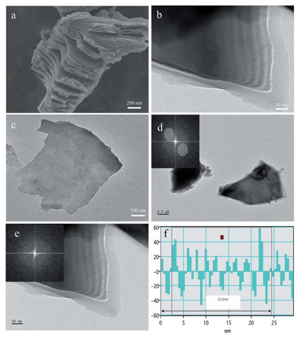
Fig. 2 (a) SEM images of layered TiVCT<sub>x</sub>. (b and c) TEM images of TiVCT<sub>x</sub>. (d-f) The interlayer analysis of TiVCT<sub>x</sub>.
