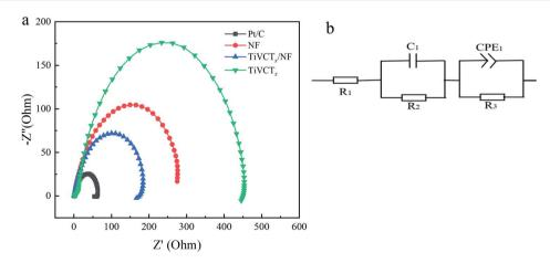
Fig. 8 (a) Electrochemical impedance spectra of Pt/C, NF, TiVCT<sub>x</sub> and TiVCT<sub>x</sub>@NF for the electrocatalytic HER at an overpotential of open-circuit potential. (b) Equivalent circuit diagram of the TiVCT<sub>x</sub>@NF composites.
