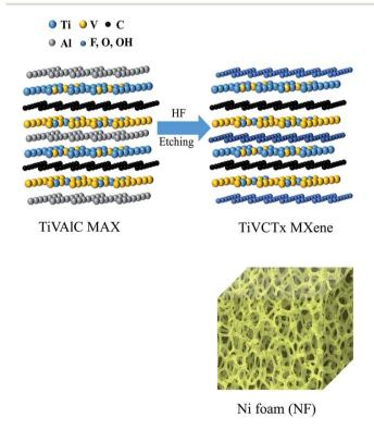
Fig. 1 Schematic illustration of the synthetic process of TiVCT<sub>x</sub>@NF.
