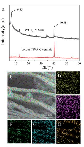
Fig. 3 (a) XRD patterns of the  $TiVCT_x$  MXene and TiVAlC powder. (b) Elemental mapping images of layered  $TiVCT_x$  nanosheets.
