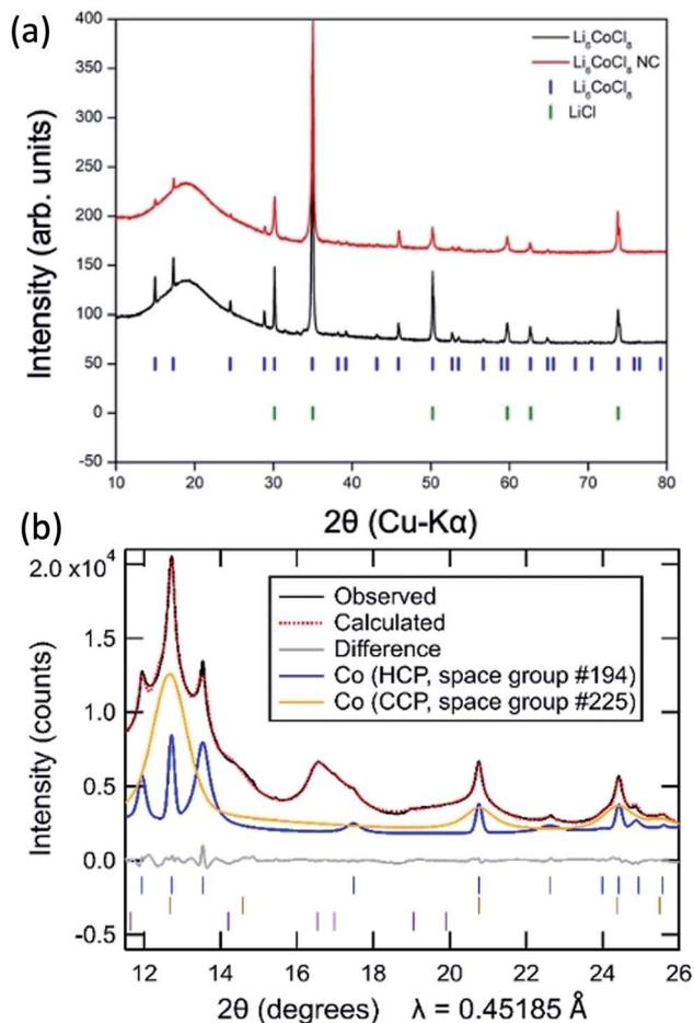
Fig. 2 (a) Laboratory XRD patterns of synthesized  $\text{Li}_6\text{CoCl}_8$  (black) and nanocomposite (red) with markers of literature peak positions of  $\text{Li}_6\text{CoCl}_8$  (blue) and LiCl (green). (b) Synchrotron diffraction pattern of Co NWs (black) with the simulated pattern (red) of an hcp (26%, blue) and ccp (74%, orange) Co mixture. Markers are shown for six minor unindexed peaks (purple), with further details in Fig. S4.†
