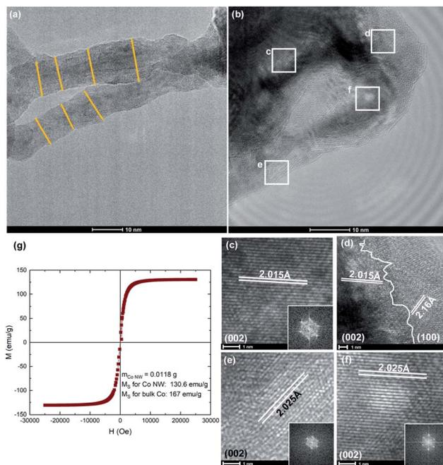
Fig. 4 Clockwise from top left: lower resolution TEM micrograph of Co NWs shows an average NW diameter of  $\sim 11$  nm (a); higher resolution TEM micrographs of Co NWs (b) with SAED insets of regions showing predominantly hcp phase (c–f) as well as the intersection of grains (d). Magnetic measurements show the  $M_s$  of NWs is close to the value of bulk cobalt value (g).
