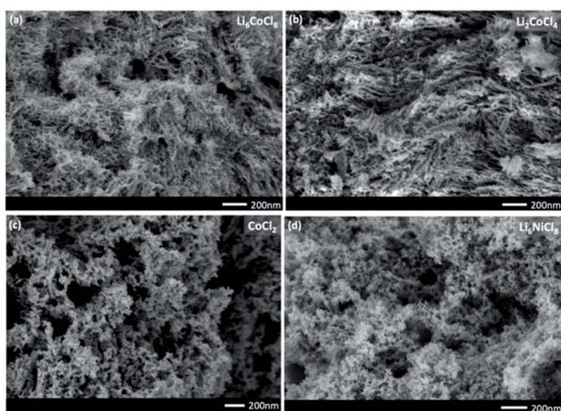
Fig. 5 SEM images comparing the effect of different precursors:  $\text{Li}_6\text{CoCl}_8$  and  $\text{Li}_2\text{CoCl}_4$  produce NWs (a and b), however less dilution ((c),  $\text{CoCl}_2$ ) and a different ccp metal ((d),  $\text{Li}_6\text{NiCl}_8$ ) lead to nanoporous morphology.
