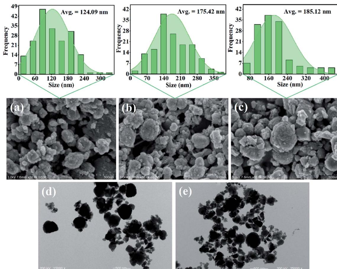
Fig. 4 SEM images of the magnetic (a) Fe<sub>3</sub>O<sub>4</sub> NPs, (b) Fe<sub>3</sub>O<sub>4</sub>/TA/PEI carrier, and (c) immobilized Alcalase. TEM images of magnetic (d) Fe<sub>3</sub>O<sub>4</sub> NPs and (e) immobilized Alcalase.
