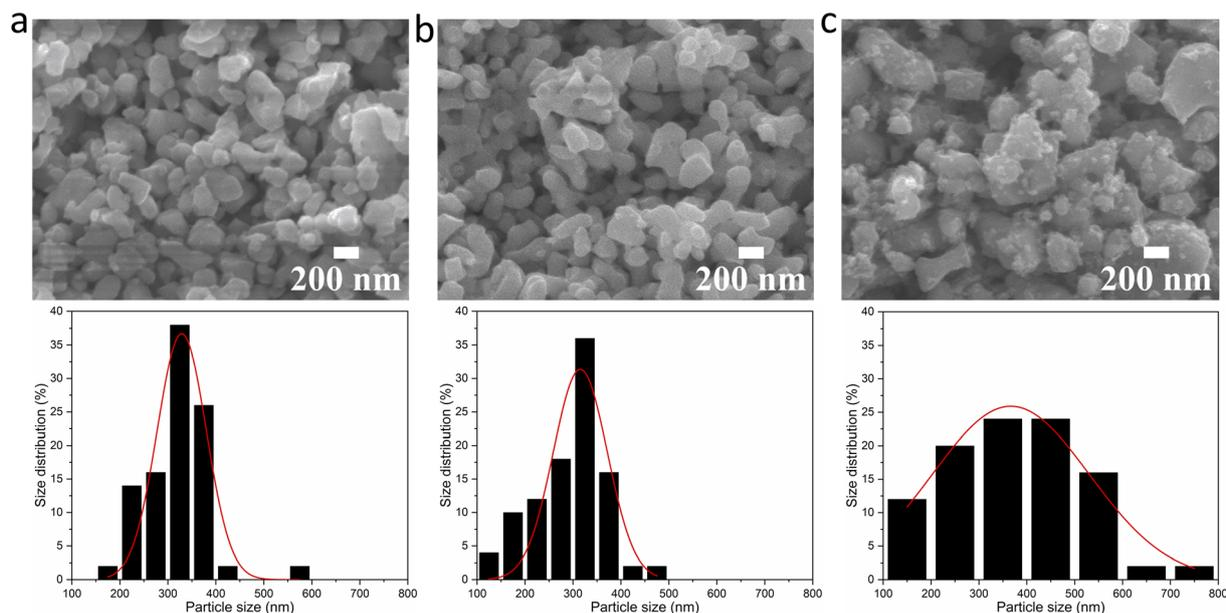
Fig. 6 SEM images of BaTiO<sub>3</sub> samples hydrothermally synthesised at 220 °C using Ba/Ti precursor ratios of (a) 4 : 1, (b) 2 : 1 and (c) 1 : 1; the patterns below to show the grain sizes of the samples determined using the ImageJ software, and the size distributions analysed with a Gaussian function.
