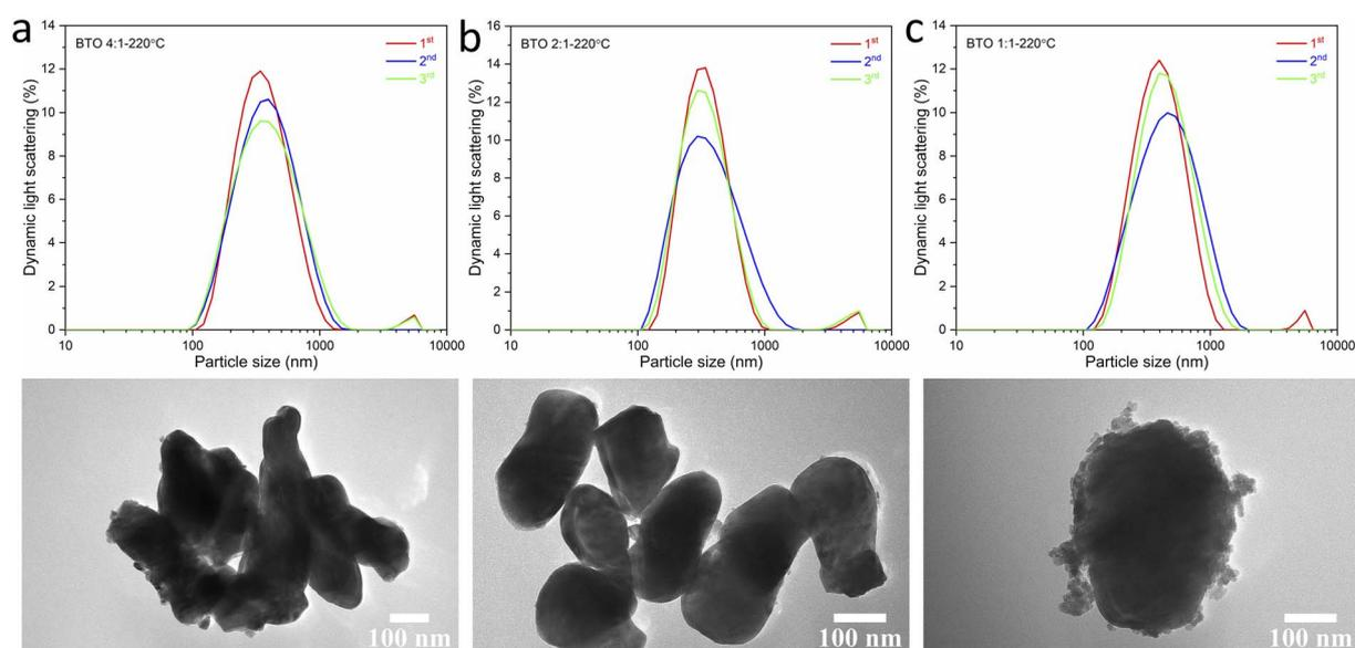
Fig. 7 DLS patterns (above) and TEM images (below) of BaTiO<sub>3</sub> samples hydrothermally synthesised at 220 °C using Ba/Ti precursor ratios of (a) 4 : 1, (b) 2 : 1 and (c) 1 : 1.
