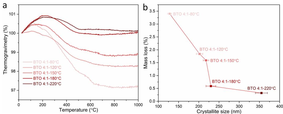
Fig. 5 (a) TGA curves and (b) mass losses against crystallite sizes of BaTiO<sub>3</sub> samples hydrothermally synthesised using a 4 : 1 Ba/Ti precursor ratio with reaction temperatures of 80, 120, 150, 180 and 220 °C, examined by heating in Ar with a heating process of at 1 °C min<sup>-1</sup> from 25 to 200 °C, then at 10 °C min<sup>-1</sup> from 200 to 1000 °C (sample labels explained in Table 1).
