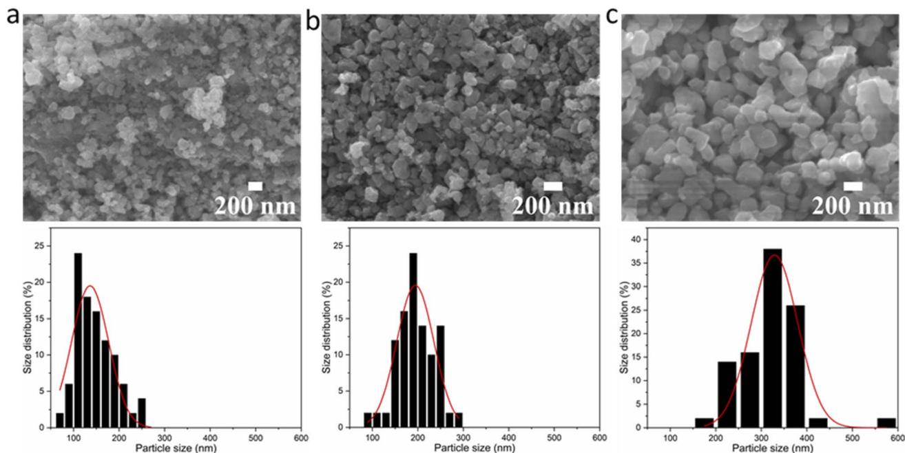
Fig. 3 SEM images of BaTiO<sub>3</sub> samples hydrothermally synthesised using a 4 : 1 Ba/Ti precursor ratio with reaction temperatures of (a) 80 °C, (b) 150 °C and (c) 220 °C; the patterns below to show the grain sizes of the samples determined using the ImageJ software, and the size distributions analysed with a Gaussian function.
