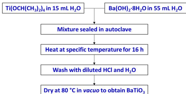
Scheme 1 Hydrothermal synthesis to prepare BaTiO<sub>3</sub>, using various Ba/Ti precursor ratios/concentrations and reaction temperatures.
