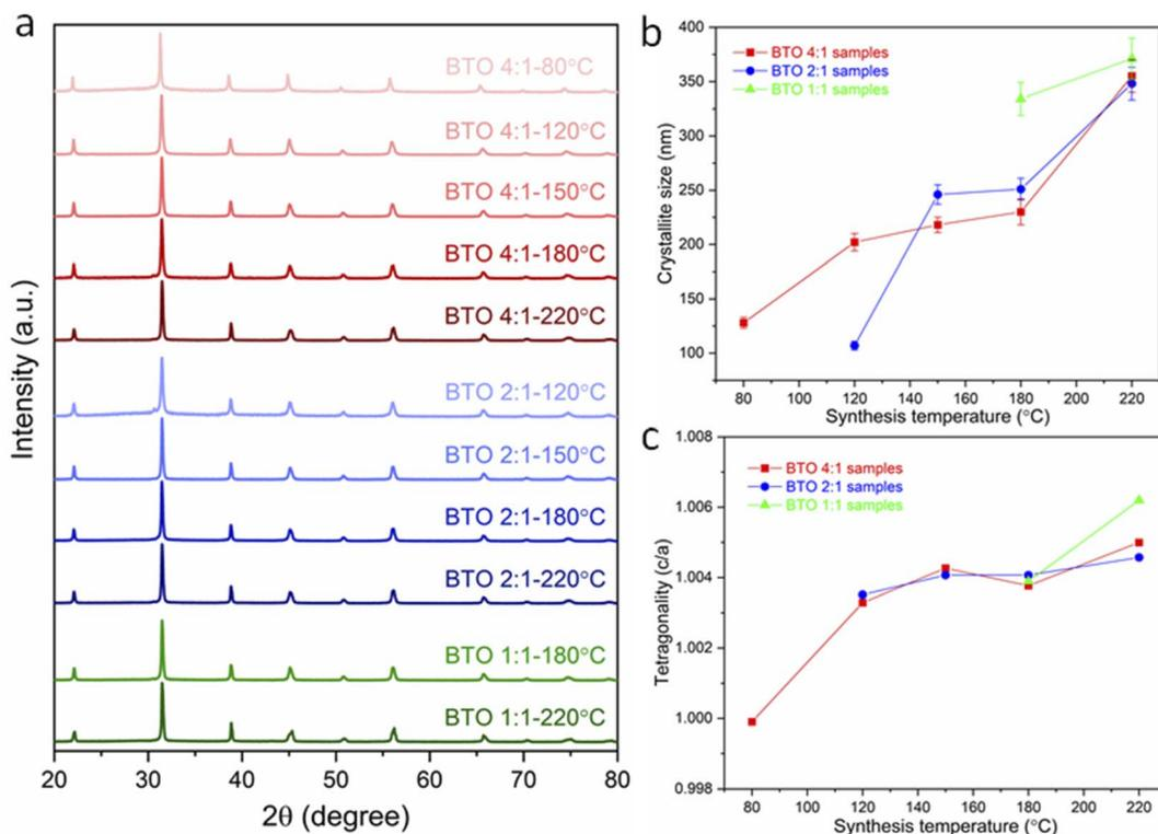
**Fig. 1** (a) XRD patterns of BaTiO<sub>3</sub> samples hydrothermally synthesised with Ba/Ti precursor ratios of 4 : 1, 2 : 1 and 1 : 1, at various reaction temperatures of 80, 120, 150, 180 and 220 °C; (b) crystallite size and (c) tetragonality ( $c/a$ ) of BaTiO<sub>3</sub> samples plotted against reaction temperature in hydrothermal synthesis using Ba/Ti precursor ratios of 4 : 1, 2 : 1 and 1 : 1, obtained from the Rietveld fits to the XRD patterns (sample labels explained in Table 1).
