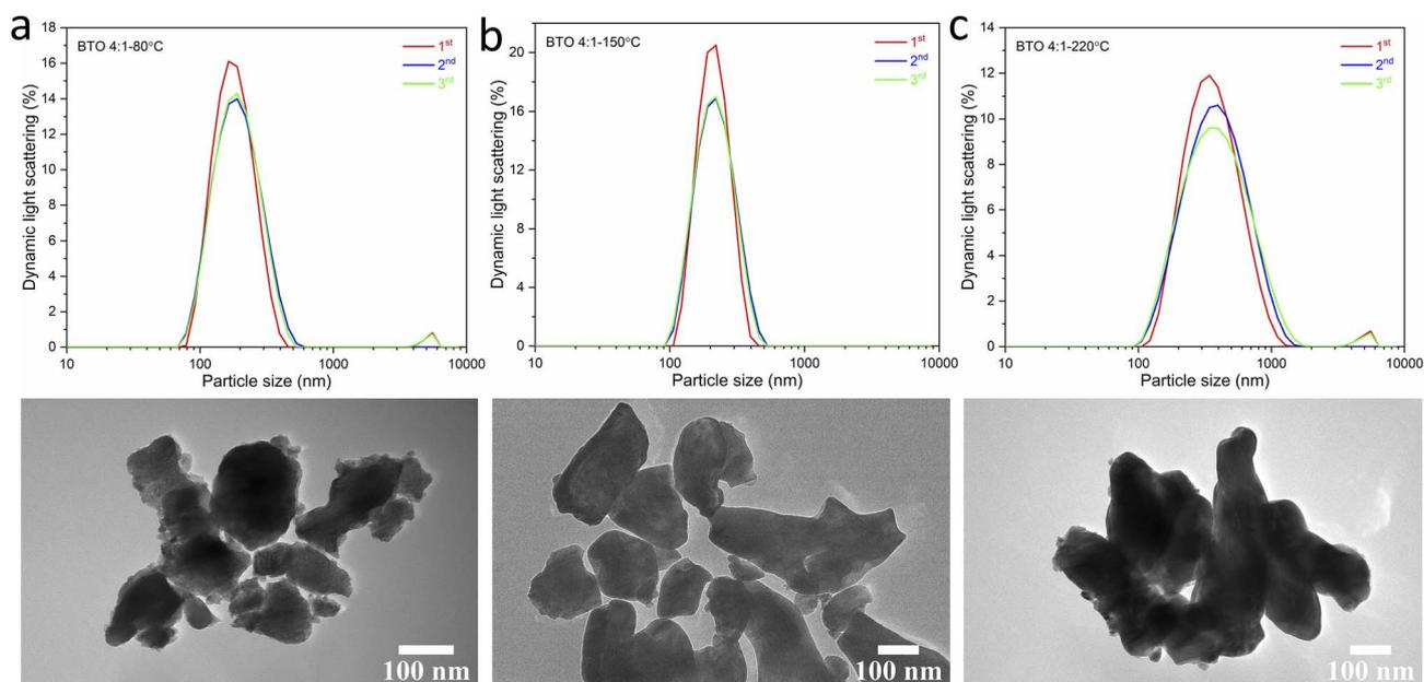
Fig. 4 DLS patterns (above) and TEM images (below) of BaTiO<sub>3</sub> samples hydrothermally synthesised using a 4 : 1 Ba/Ti precursor ratio with reaction temperatures of (a) 80 °C, (b) 150 °C and (c) 220 °C.
