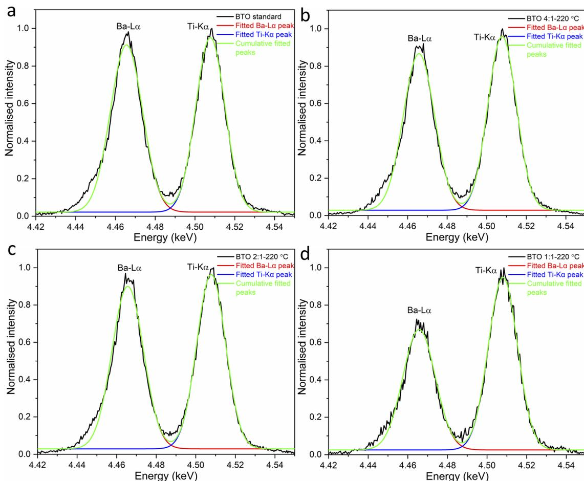
Fig. 8 Fit of the WDS spectra peaks for the Ba–L $\alpha$  and Ti–K $\alpha$  peaks of (a) the standard BaTiO $_3$  and BaTiO $_3$  samples hydrothermally synthesised at 220 °C using Ba/Ti precursor ratios of (b) 4 : 1, (c) 2 : 1 and (d) 1 : 1 (sample labels explained in Table 1).
