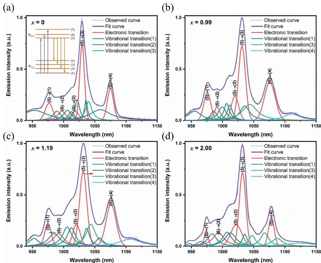
Fig. 6 Decomposed fluorescence spectra at room temperature with different contents. (a)  $x = 0$ , (b)  $x = 0.99$ , (c)  $x = 1.19$ , and (d)  $x = 2.00$ . The electronic transition peaks have been identified as the transitions from the  ${}^2F_{5/2}$  energy levels (5)–(7) to the four  ${}^2F_{7/2}$  energy levels (1)–(4). The vibrational transitions ( $i$ ) corresponding to the phonon sidebands of (5)–( $i$ ), ( $i = 1, 2, 3$ , and 4) energy levels transitions, respectively.
