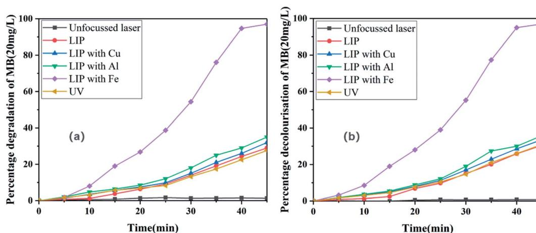
Fig. 3 (a) Degradation and (b) decolourisation of MB dye (20 mg L<sup>-1</sup>) in the presence of different sources of light irradiation.
