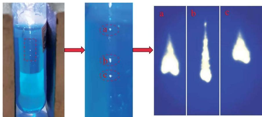
Fig. 4 Plasma in MB excited with laser pulses.
