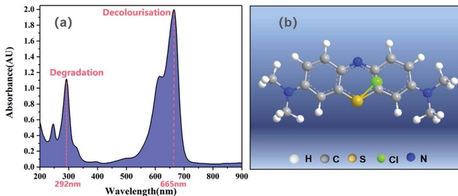
Fig. 1 (a) UV-vis spectra of methylene blue (MB) and (b) its structural formula.<sup>12</sup>
