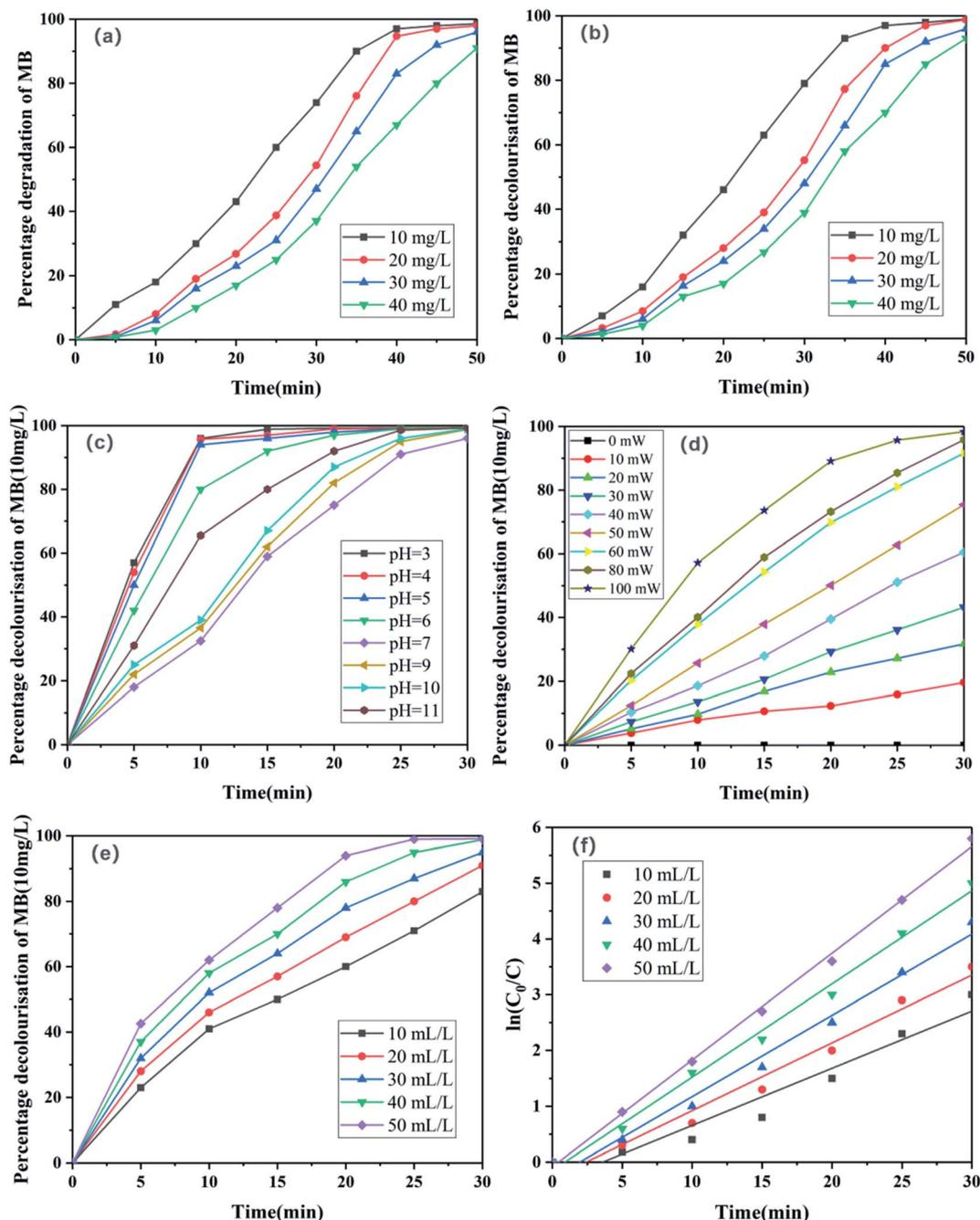
Fig. 8 Effects of MB concentration on its (a) degradation and (b) decolourisation. (c) Effects of pH on decolourisation of MB. (d) Effects of laser energy on decolourisation of MB. (e) Effects of initial H<sub>2</sub>O<sub>2</sub> concentration on MB degradation and (f) linear plots of ln(C<sub>0</sub>/C) for the photo-degradation of MB under LIP excitation of Fe sheet.
