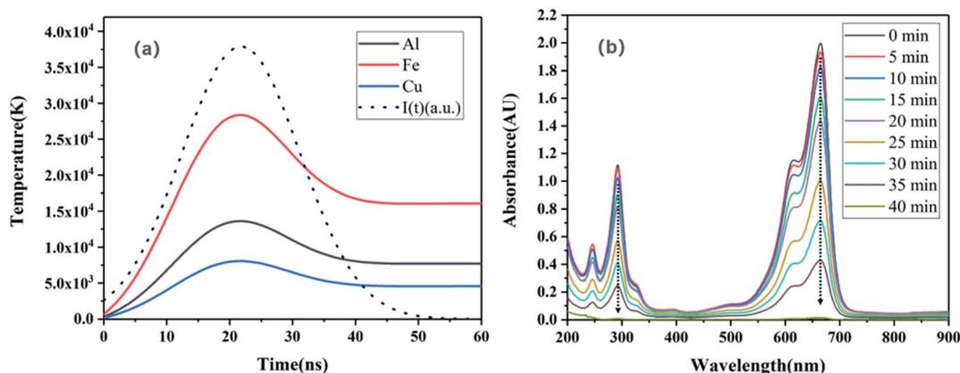
Fig. 6 (a) Transient surface temperature profiles derived using the heat diffusion model. The dashed line indicates the incident intensity  $I(t)$  (arbitrary scale). (b) Typical absorbance spectra of MB dye after treatment with Fe under LIP irradiation.
