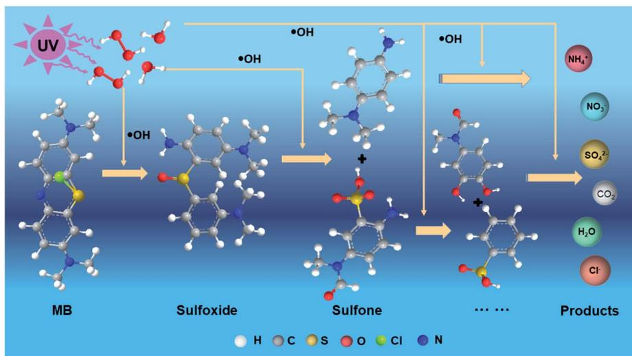
Fig. 7 Schematic diagram of photodegradation of MB.
