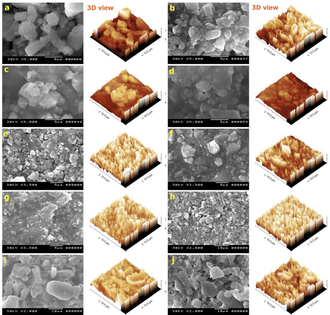
Fig. 2 SEM micrographs of HA/CS composite coated specimens in the mixture at 30 V and deposition time of 10 min, with different PVB concentrations (a) without PVB, (b)  $0.25 \text{ g L}^{-1}$  PVB, (c)  $0.5 \text{ g L}^{-1}$  PVB, (d)  $1 \text{ g L}^{-1}$  PVB, (e)  $0.25 \text{ g L}^{-1}$  PEG, (f)  $0.5 \text{ g L}^{-1}$  PEG, (g)  $1 \text{ g L}^{-1}$  PEG, (h)  $2 \text{ mL L}^{-1}$  TEA, (i)  $4 \text{ mL per L TEA}$  and (j)  $10 \text{ mL L}^{-1}$  TEA.
