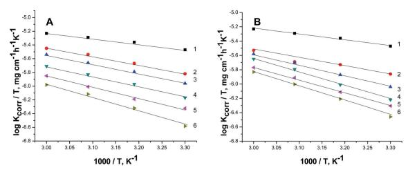
Fig. 8 Plots of log  $K_{corr.}/T$  versus 1/T for S-Fe in the free 1 M HCl solution and in the presence of different concentrations of (A) PS and (B) PBT compounds: (1) 0.0, (2) 100, (3) 200, (4) 300, (5) 400, (6) 500 mg l<sup>-1</sup>.
