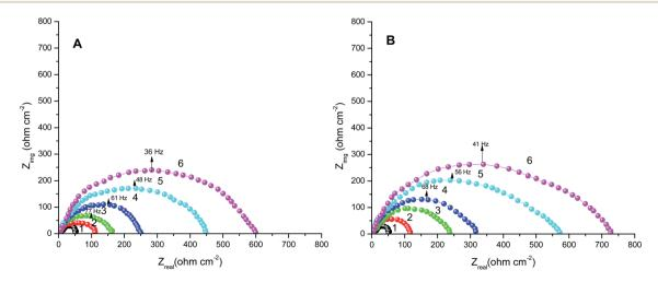
Fig. 3 Nyquist plots for S-Fe corrosion in the blank 1.0 M HCl solution and when containing different concentrations of (A) PS and (B) PBT at 300 K: (1) 0.0, (2) 100, (3) 200, (4) 300, (5) 400, (6) 500 mg  $l^{-1}$ .
