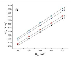
Fig. 9 Langmuir adsorption isotherms for S-Fe in the blank 1 M HCl solution and in the presence of different concentrations of (A) PS and (B) PBT compounds at: (1) 303 K, (2) 313 K, (3) 323 K, (4) 333 K.
