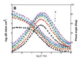
Fig. 4 Bode plots for S-Fe corrosion in the blank 1.0 M HCl solution and when containing different concentrations of (A) PS and (B) PBT at 300 K: (1) 0.0, (2) 100, (3) 200, (4) 300, (5) 400 m (6) 500 mg  $l^{-1}$ .
