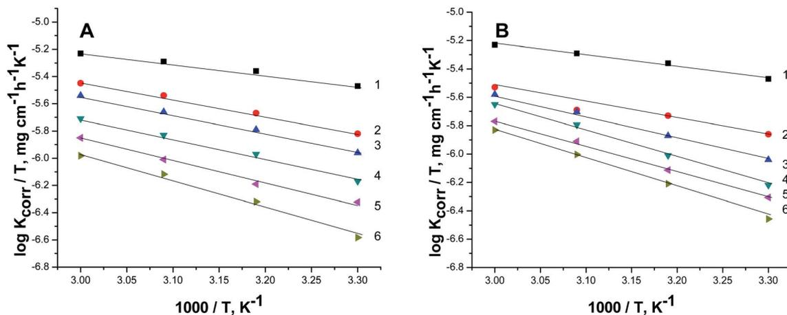
Fig. 8 Plots of  $\log K_{\text{corr}}/T$  versus  $1/T$  for S-Fe in the free 1 M HCl solution and in the presence of different concentrations of (A) PS and (B) PBT compounds: (1) 0.0, (2) 100, (3) 200, (4) 300, (5) 400, (6) 500  $\text{mg l}^{-1}$ .
