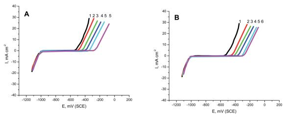
Fig. 5 PDAP curves of S-Fe corrosion in the free 1.0 M HCl + 0.5 M NaCl solution and when containing different concentrations of (A) PS and (B) PBT at 300 K at a scan rate of 0.2 mV s<sup>-1</sup>: (1) 0.0, (2) 100, (3) 200, (4) 300, (5) 400, (6) 500 mg l<sup>-1</sup>.
