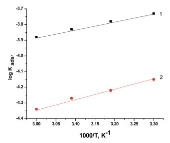
Fig. 10 Plots of log  $K_{\rm ads}$  versus 1000/T for the corrosion of S-Fe in 1.0 M HCl solution in the presence of PS and PBT compounds at different temperatures: (1) PBT and (2) PS.
