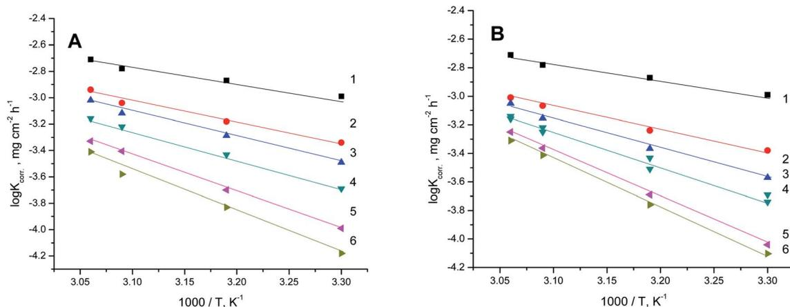
Fig. 7 Plots of  $\log K_{\text{corr.}}$  versus  $1/T$  for S-Fe in the free 1 M HCl solution and in the presence of different concentrations of (A) PS and (B) PBT compounds. (1) 0.0, (2) 100, (3) 200, (4) 300, (5) 400, (6) 500  $\text{mg l}^{-1}$ .
