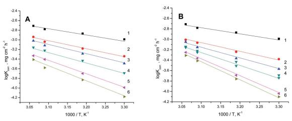
Fig. 7 Plots of log  $K_{corr.}$  versus 1/T for S-Fe in the free 1 M HCl solution and in the presence of different concentrations of (A) PS and (B) PBT compounds. (1) 0.0, (2) 100, (3) 200, (4) 300, (5) 400, (6) 500 mg l<sup>-1</sup>.
