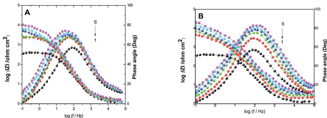
**Fig. 4** Bode plots for S-Fe corrosion in the blank 1.0 M HCl solution and when containing different concentrations of (A) PS and (B) PBT at 300 K: (1) 0.0, (2) 100, (3) 200, (4) 300, (5) 400 m (6) 500 mg l<sup>-1</sup>.
