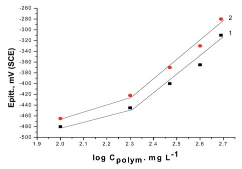
Fig. 6 Relationship between Epitt and the logarithmic concentrations of the two polymer compounds: (1) PS and (2) PBT.
