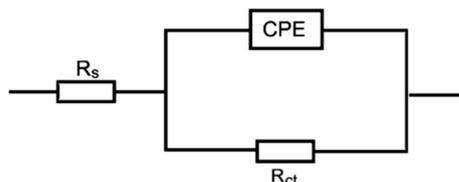
Fig. 2 Electrochemical equivalent circuit applied to fit the EIS measurements.
