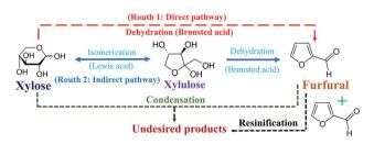
Fig. 3 Direct and indirect pathways of furfural production from xylose.
