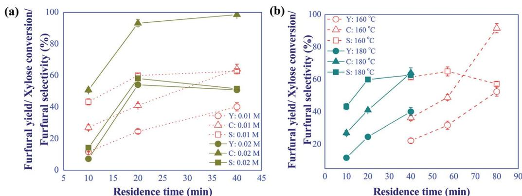
Fig. 4 (a) Effects of formic acid concentration (conditions; xylose: 10 g L<sup>-1</sup> and temp: 180 °C) and (b) reaction temperature (conditions; FA: 10 mM and xylose: 10 g L<sup>-1</sup>) on the furfural yield (Y)/selectivity (S) and xylose conversion (C) under various residence times.
