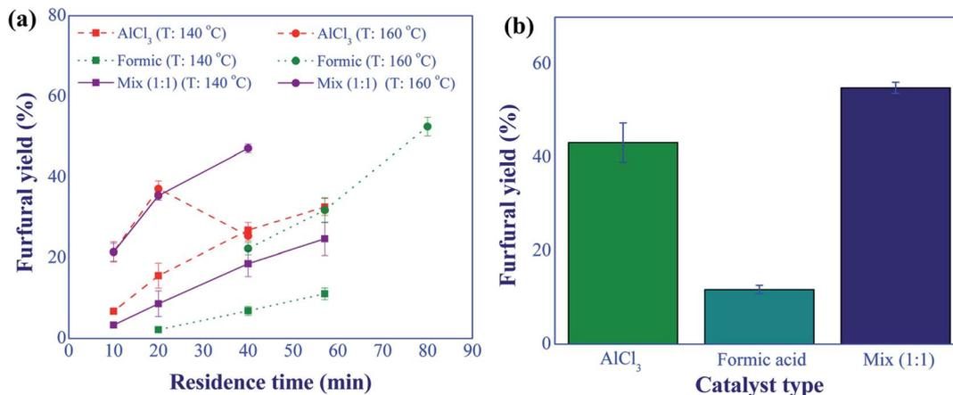
Fig. 7 Furfural yield comparison between the uses of individual catalyst and dual catalysts; (a) at 140 and 160 °C with various residence times, (b) at 180 °C and 10 min (conditions; catalyst: 10 mM and xylose: 10 g L<sup>-1</sup>).
