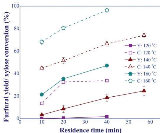
Fig. 8 Effects of residence times and temperatures on the furfural yield (Y) and xylose conversion (C), synthesized under the dual-acid catalysts (condition: AlCl<sub>3</sub>-to-FA: 1 : 1, total catalyst: 10 mM).
