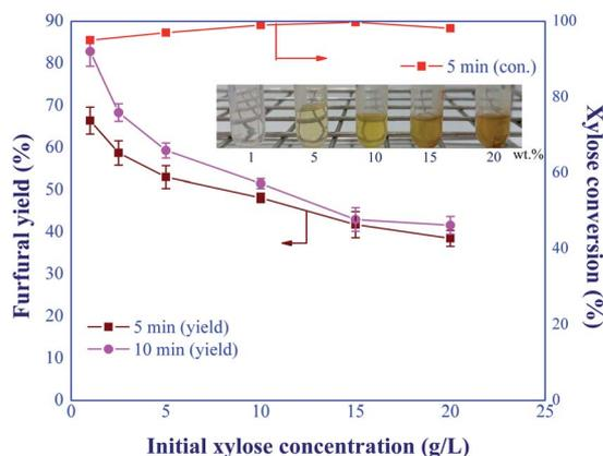
Fig. 11 Effect of initial xylose concentrations on the furfural yield under the various residence times (condition: AlCl<sub>3</sub>-to-FA: 1 : 1, total catalyst: 20 mM, temp: 180 °C).
