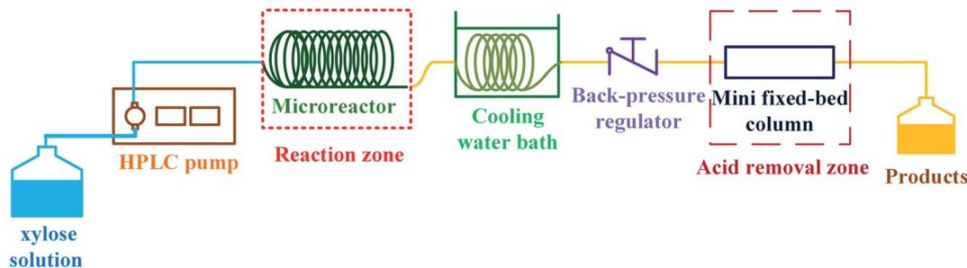
Fig. 2 Proposed continuous furfural production with acid catalyst removal.
