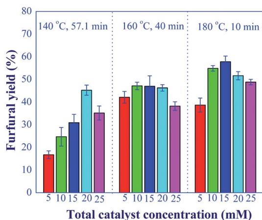
Fig. 10 Effect of total catalyst amounts on the furfural yield under the various conditions; 140 °C and 57.1 min; 160 °C and 40 min; 180 °C and 10 min (condition AlCl<sub>3</sub>-to-FA: 1 : 1).
