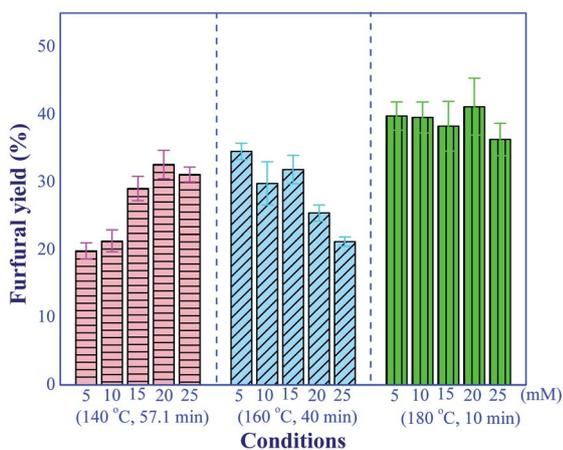
Fig. 6 Effect of aluminum chloride concentrations on the furfural yield under the various operating conditions (conditions; xylose: 10 g L<sup>-1</sup>).
