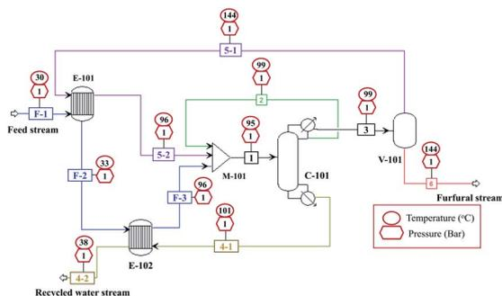
Fig. 13 Conceptual design of furfural purification process (heat exchangers (E101–E102), flash drum (V-101), distillation tower (C-101), and mixer (M-101)).
