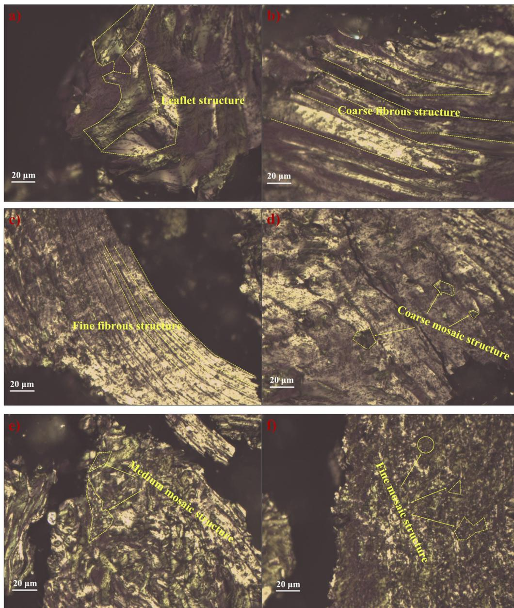
Fig. 5 Typical optical microstructure of needle cokes: leaflet structure (a), coarse fibrous structure (b), fine fibrous structure (c), coarse mosaic structure (d), medium coarse structure (e), and fine mosaic structure (f).
