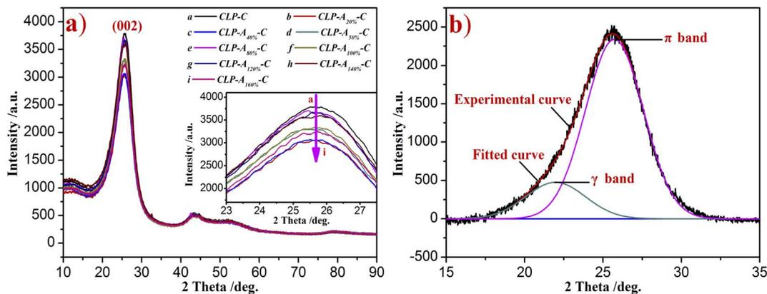
Fig. 6 XRD patterns of needle coke (a) and curve-fitted graph of CLP-A<sub>20%</sub>-C (b).
