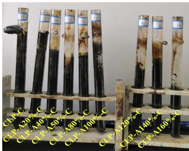
Fig. 4 Optical images of the produced needle coke.
