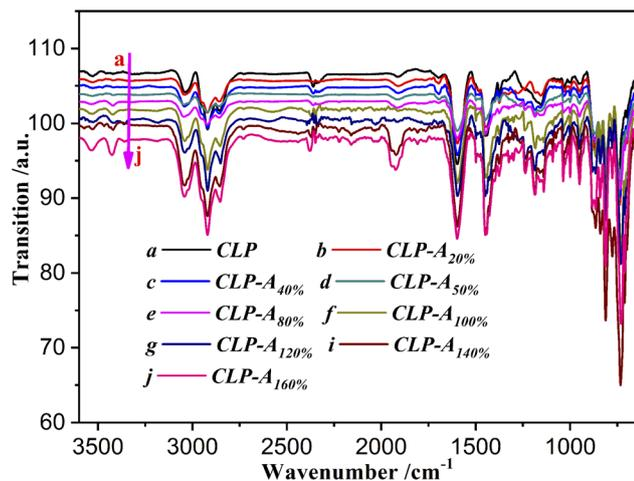
Fig. 2 FTIR spectra of the blending pitches.
