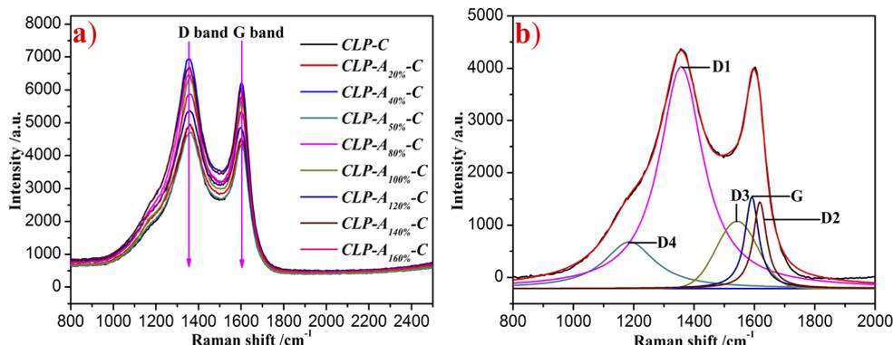
Fig. 7 Raman spectra of needle cokes (a) and curve-fitted graph of CLP-A<sub>20%</sub>-C (b).
