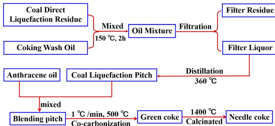
Fig. 1 Flow diagram of the preparation process of needle coke.
