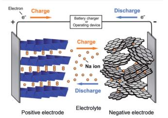
Fig. 5 Schematic showing the working principle of the sodium ion battery. (Adapted from ref. 31, copyright 2014 American Chemical Society).
