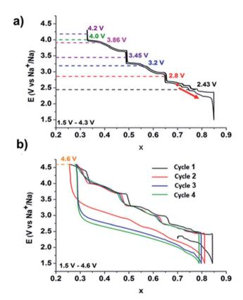
Fig. 20 Galvanostatic cycling curve of a Na//P2-Na<sub>x</sub>CoO<sub>2</sub> battery representing the phase diagram. (Adapted with permission from ref. 93, copyright 2022 American Chemical Society)
