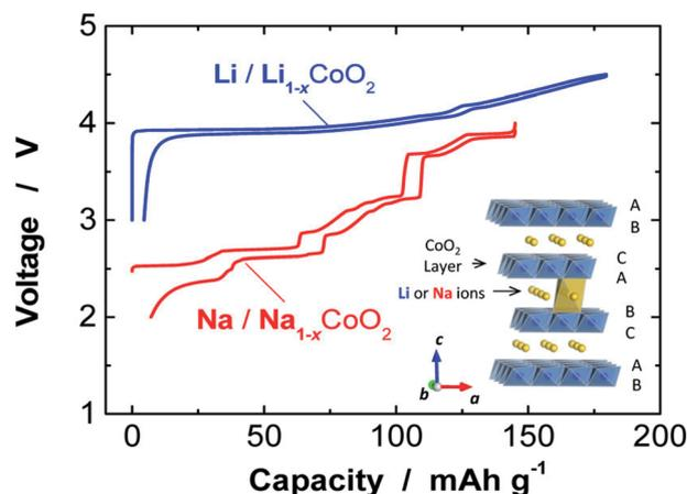
Fig. 4 Comparison of charge/discharge plots of Na/NaCoO<sub>2</sub> and Li/LiCoO<sub>2</sub> cells. (Adapted from ref. 31, copyright 2014 American Chemical Society).
