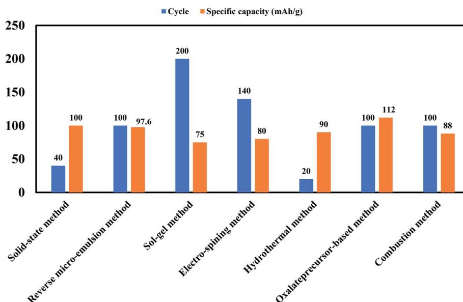
Fig. 8 Bar chart showing comparison of specific capacity and cycle number for material  $\text{Na}_{0.44}\text{MnO}_2$  made by various processes as cathodes for sodium-ion batteries.
