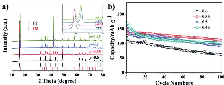
Fig. 18 (a) XRD patterns of  $\text{Na}_{0.8}\text{Mn}_y\text{Ni}_{0.8-y}\text{Fe}_{0.1}\text{Ti}_{0.1}\text{O}_2$  ( $y = 0.45, 0.5, 0.55, 0.6$ ). (b) Cycling performance of  $\text{Na}_{0.8}\text{Mn}_y\text{Ni}_{0.8-y}\text{Fe}_{0.1}\text{Ti}_{0.1}\text{O}_2$  ( $y = 0.45, 0.5, 0.55, 0.6$ ). (Adapted from ref. 90, copyright 2021 Royal Society of Chemistry).
