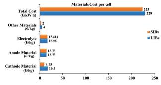
Fig. 2 Evaluation of the fabrication costs for LIB and SIB.<sup>21</sup>
