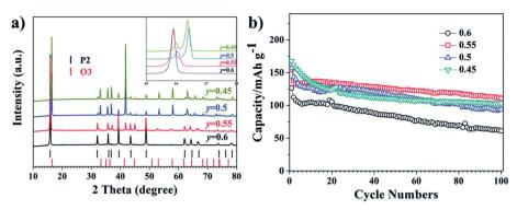
Fig. 18 (a) XRD patterns of  $Na_{0.8}Mn_yNi_{0.8-y}Fe_{0.1}Ti_{0.1}O_2$  (y = 0.45, 0.5, 0.55, 0.6). (b) Cycling performance of  $Na_{0.8}Mn_yNi_{0.8-y}Fe_{0.1}Ti_{0.1}O_2$  (y = 0.45, 0.5, 0.55, 0.6). (Adapted from ref. 90, copyright 2021 Royal Society of Chemistry).
