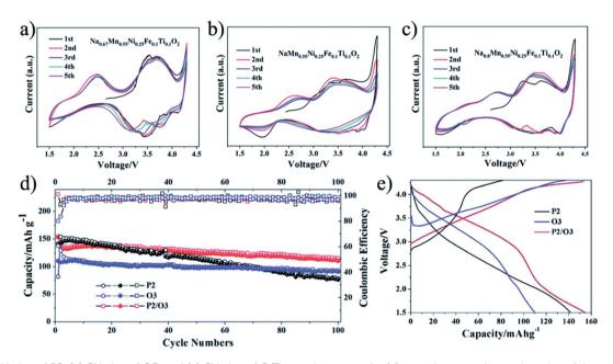
Fig. 17 (a) CV plot of P2, (b) CV plot of O3, and (c) CV plot of O/P two phase sample; (d) capacity vs. cycle number plot of the samples and (e) voltage-first discharge capacity plots. (Adapted from ref. 90, copyright 2021 Royal Society of Chemistry).
