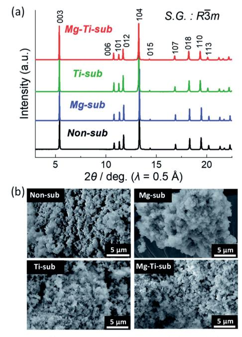
Fig. 9 (a) X-ray diffraction patterns and (b) SEM images of pristine  $Na[Ni_{4/9}Mn_{1/3}Mg_{1/18}Ti_{1/6}]O_2$  (Mg-Ti-sub),  $Na[Ni_{1/2}Mn_{1/2}]O_2$  (non-sub),  $Na[Ni_{4/9}Mn_{1/2}Mg_{1/18}]O_2$  (Mg-sub) and  $Na[Ni_{1/2}Mn_{1/3}Ti_{1/6}]O_2$  (Ti-sub). (Adapted from ref. 59, copyright 2021 Royal Society of Chemistry).
