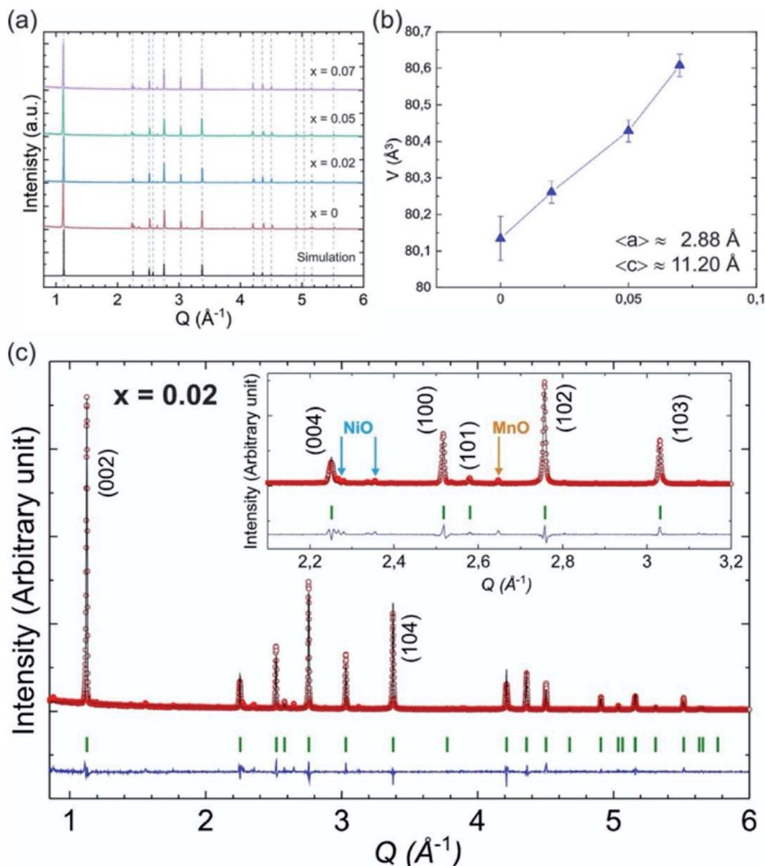
Fig. 12 (a) XRD pattern of P2-type  $\text{Na}_{0.5}\text{Mn}_{0.83}\text{Mg}_x\text{Ni}_{0.17-x}\text{O}_2$  ( $x = 0.07, 0.05, 0.02$  and  $0$ ) samples together with a simulated pattern based on  $x = 0$  structure. (b) Cell volume for different Mg content ( $x$ ) along with the average lattice parameters  $\langle a \rangle$  and  $\langle c \rangle$ . (c) Rietveld refinement of the XRD data for the  $x = 0.02$  sample. (Adapted from ref. 72, copyright 2021 Royal Society of Chemistry).
