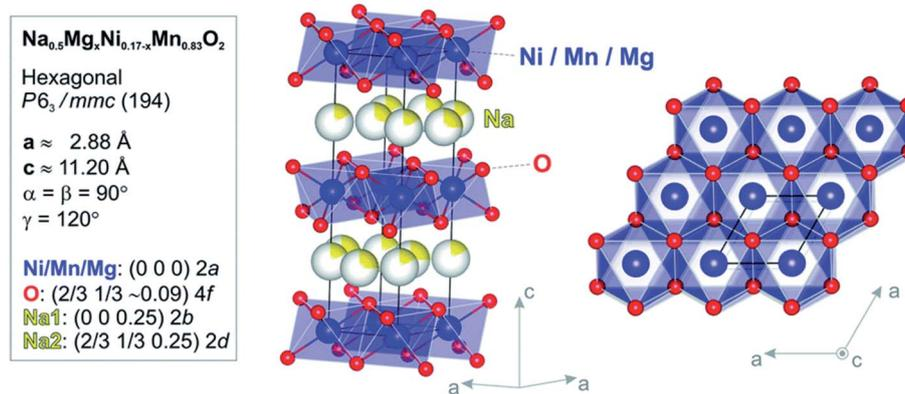
Fig. 14 Model of atomic structure (side-view and top-view) and the atomic positions and crystallographic constraints for  $\text{Na}_{0.5}\text{Mn}_{0.83}\text{Mg}_x\text{-Ni}_{0.17-x}\text{O}_2$  calculated by Rietveld refinement study of the RTXRD pattern based on the structure of  $x = 0$  sample. (Adapted from ref. 72, copyright 2021 Royal Society of Chemistry).
