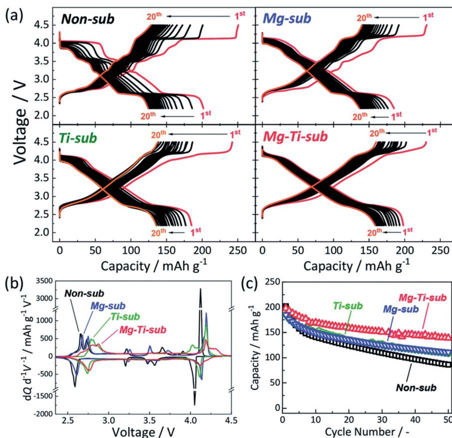
Fig. 10 (a) Galvanostatic charge–discharge plot, (b) dQ/dV plot, and (c) cyclic stability of Mg–Ti-sub, non-sub, Mg-sub and Ti-sub and electrodes in Na-ion cells. At 12 mA g<sup>-1</sup> current density galvanostatic charge–discharge experiments were conducted. (Adapted from ref. 60, copyright 2021 Royal Society of Chemistry).
