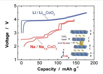
Fig. 4 Comparison of charge/discharge plots of Na/NaCoO $_2$  and Li/LiCoO $_2$  cells. (Adapted from ref. 31, copyright 2014 American Chemical Society).
