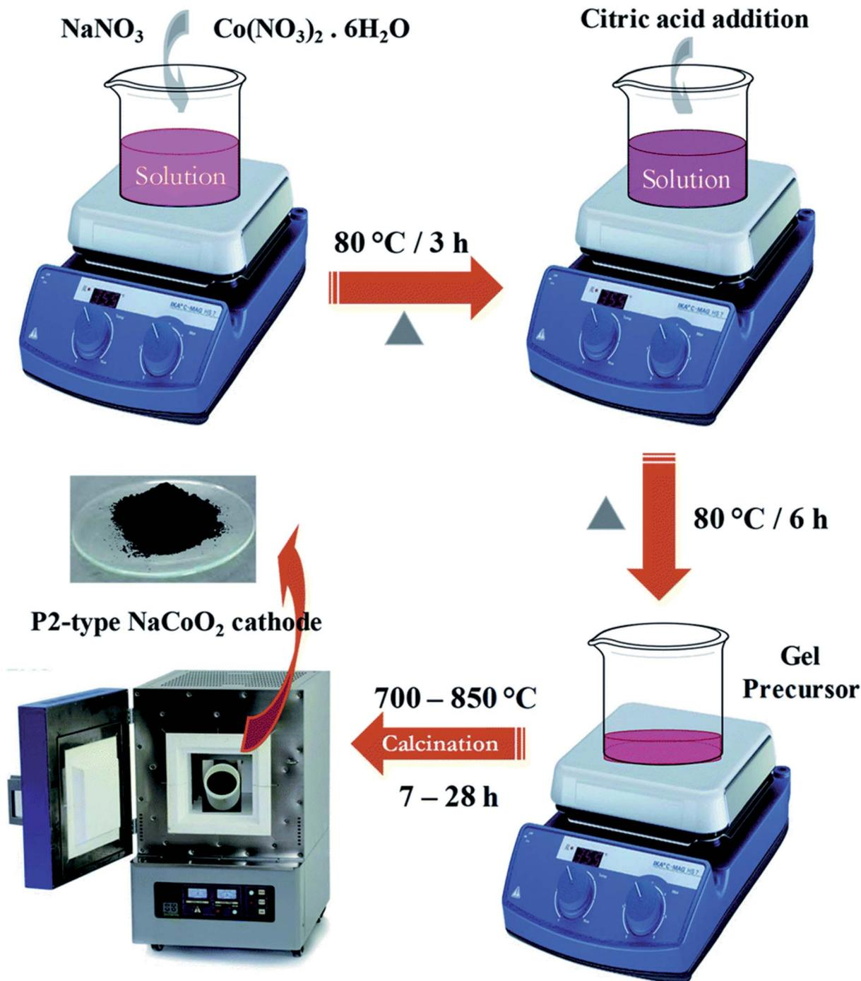
Fig. 23 Synthesis scheme of the NaCoO<sub>2</sub> cathode. (Adapted from ref. 163, copyright 2021 Royal Society of Chemistry).
