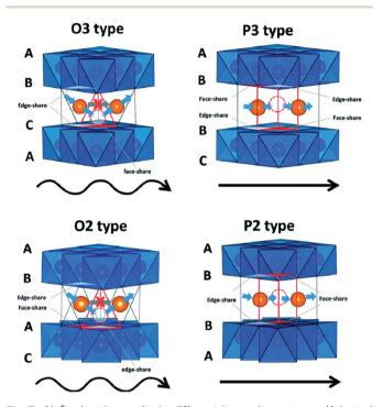
Fig. 7 Na<sup>+</sup> migration paths in different layered structures. (Adapted from ref. 31, copyright 2014 American Chemical Society).
