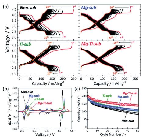
Fig. 10 (a) Galvanometric charge–discharge plot, (b) dQ/dV plot, and (c) cyclic stability of Mg–Ti-sub, non-sub, Mg-sub and Ti-sub and electrodes in Na-ion cells. At 12 mA  $g^{-1}$  current density galvanostatic charge–discharge experiments were conducted. (Adapted from ref. 60, copyright 2021 Royal Society of Chemistry).
