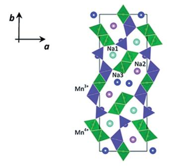
Fig. 22 Crystal structure of tunnel-type Na<sub>0.44</sub> MnO<sub>2</sub>. (Adapted with the permission from ref. 103, copyright 2022 Royal Society of Chemistry)
