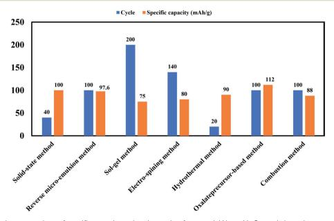
Fig. 8 Bar chart showing comparison of specific capacity and cycle number for material Na<sub>0.44</sub>MnO<sub>2</sub> made by various processes as cathodes for sodium-ion batteries.
