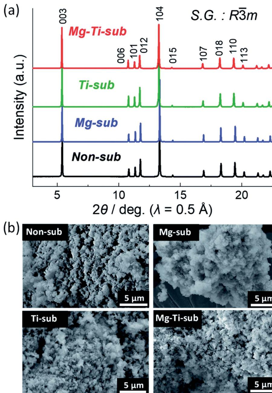
Fig. 9 (a) X-ray diffraction patterns and (b) SEM images of pristine  $\text{Na}[\text{Ni}_{4/9}\text{Mn}_{1/3}\text{Mg}_{1/18}\text{Ti}_{1/6}]\text{O}_2$  (Mg–Ti-sub),  $\text{Na}[\text{Ni}_{1/2}\text{Mn}_{1/2}]\text{O}_2$  (non-sub),  $\text{Na}[\text{Ni}_{4/9}\text{Mn}_{1/2}\text{Mg}_{1/18}]\text{O}_2$  (Mg-sub) and  $\text{Na}[\text{Ni}_{1/2}\text{Mn}_{1/3}\text{Ti}_{1/6}]\text{O}_2$  (Ti-sub). (Adapted from ref. 59, copyright 2021 Royal Society of Chemistry).
