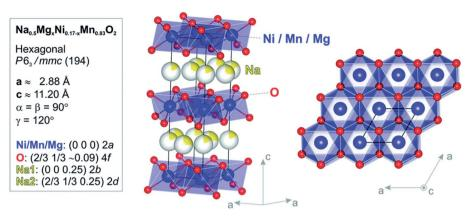
Fig. 14 Model of atomic structure (side-view and top-view) and the atomic positions and crystallographic constraints for  $Na_{0.5}Mn_{0.83}Mg_x$ - $Ni_{0.17-x}O_2$  calculated by Rietveld refinement study of the RTXRD pattern based on the structure of x=0 sample. (Adapted from ref. 72, copyright 2021 Royal Society of Chemistry).
