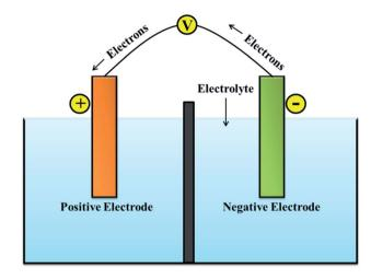
Fig. 1 Schematic of battery system.
