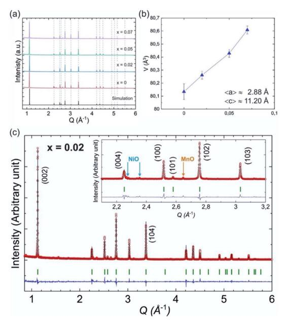
Fig. 12 (a) XRD pattern of P2-type Na<sub>0.5</sub>Mn<sub>0.83</sub>Mg<sub>x</sub>Ni<sub>0.17-x</sub>O<sub>2</sub> (x=0.07,0.05,0.02 and 0) samples together with a simulated pattern based on x=0 structure. (b) Cell volume for different Mg content (x) along with the average lattice parameters (x) and (x). (c) Rietveld refinement of the XRD data for the x=0.02 sample. (Adapted from ref. 72, copyright 2021 Royal Society of Chemistry).
