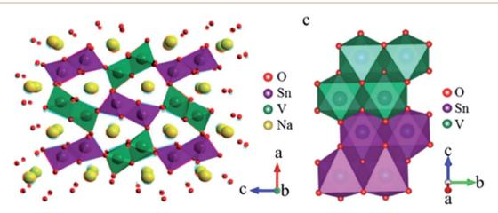
Fig. 21 Crystal structure of post-spinel NaVSnO<sub>4</sub>. (Adapted with the permission from ref. 100, copyright 2017 Wiley Online Library).
