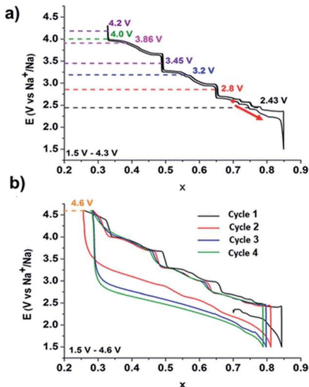
Fig. 20 Galvanostatic cycling curve of a Na//P2- $\text{Na}_x\text{CoO}_2$  battery representing the phase diagram. (Adapted with permission from ref. 93, copyright 2022 American Chemical Society).
