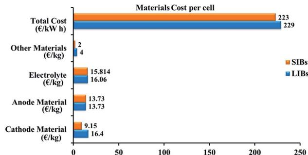
Fig. 2 Evaluation of the fabrication costs for LIB and SIB.<sup>21</sup>
