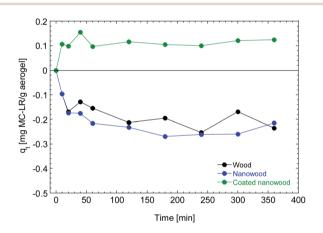
Fig. 6 Adsorption kinetic of wood, nanowood and the coated nanowood on a 5.4  $\mu g$  mL<sup>-1</sup> on a solution for 6 h.
