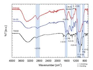
Fig. 2 FTIR-ATR spectra of the TEMPO oxidized β-cyclodextrin (TOCD), chitosan and the grafter material of both (Ch–CD). There the formation of the C–N bond is visible *ca.* 1490 cm<sup>-1</sup> as well as the reduction of the carboxyl bond at 1750 cm<sup>-1</sup> added to TOCD, confirming the reaction.
