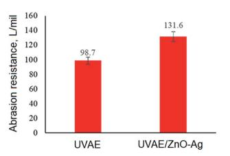
Fig. 14 Values of abrasion resistance for UV-cured UVAE and UVAE/  $\rm ZnO-Ag$  coatings.
