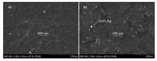
Fig. 12 FE-SEM photographs of UV-cured UVAE/ZnO-Aq in cross-section: (a) ×20 000 and (b) ×60 000.
