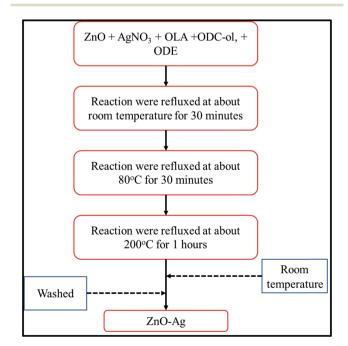
Fig. 3 Scheme for fabrication of ZnO-Ag nanohybrids.
