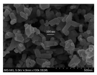
Fig. 1 FE-SEM photographs of as-received nano-ZnO.
