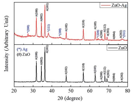
Fig. 7 XRD diffraction diagrams of ZnO-Aq nanohybrids (ZnO-Aq) and pure ZnO nanoparticles (ZnO).
