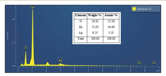
Fig. 5 EDX spectra of ZnO-Ag nanohybrids.
