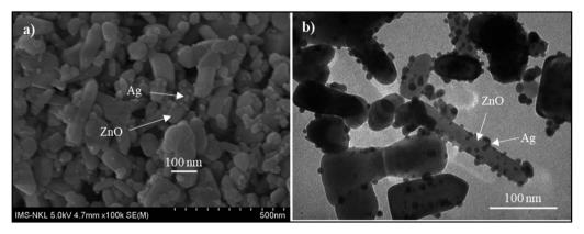
Fig. 4 FE-SEM (a) and TEM (b) photographs of ZnO-Ag nanohybrids.
