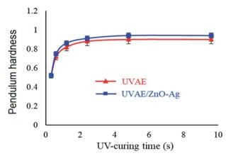
**Fig. 13** Variation of coating pendulum hardness during curing process for UVAE and UVAE/ZnO-Aq coatings.
