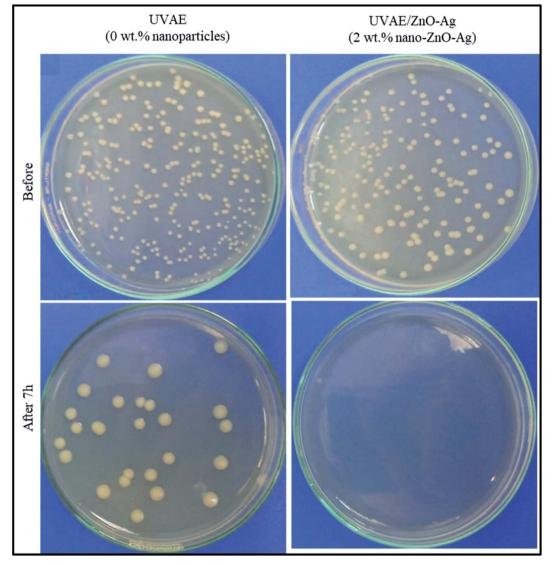
Fig. 15 Photographs of Petri dishes for antibacterial test samples.
