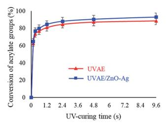
Fig. 10 Conversion of AD bonds during the UV exposure.
