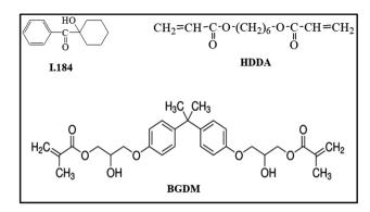
Fig. 2 Chemical formulas of I.184, HDDA and BGDM.
