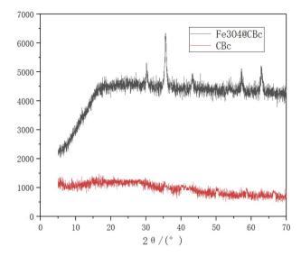
Fig. 4 XRD patterns of CBc and Fe<sub>3</sub>O<sub>4</sub>/CBc.
