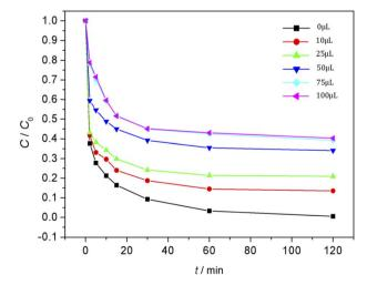
Fig. 11 Effect of t-butanol inhibitor on MO removal.
