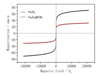
Fig. 5 Magnetization curves of CBc and Fe<sub>3</sub>O<sub>4</sub>/CBc composites.
