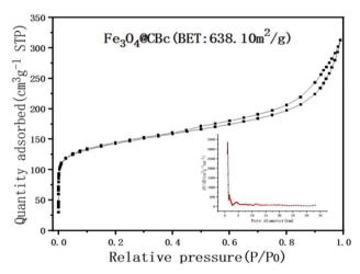
Fig. 2 Nitrogen adsorption and desorption curve and pore size distribution of CBc and  $Fe_3O_4/CBc$ .
