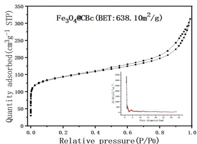
Fig. 2 Nitrogen adsorption and desorption curve and pore size distribution of Cbc and Fe<sub>3</sub>O<sub>4</sub>/Cbc.
