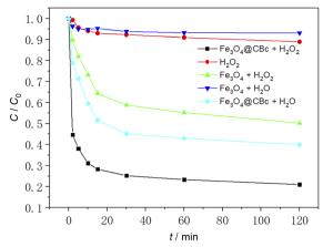
Fig. 6 Effect of different conditions on MO removal.
