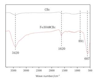
Fig. 3 FT-IR spectra of CBc and Fe<sub>3</sub>O<sub>4</sub>/CBc.
