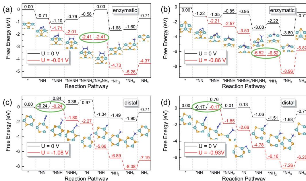
Fig. 2 Gibbs free energy diagrams of the most favorable pathway on (a) pristine zigzag edge, (b) zigzag edge with a Se vacancy, (c) pristine armchair edge, and (d) armchair edge with a Se vacancy under zero (black) and applied (red) electrode potentials. Green circles denote the potential-limiting steps. The reference potential is set to 0 V vs. the CHE. Orange, teal, blue and pink balls represent Se, Nb, N and H atoms, respectively.
