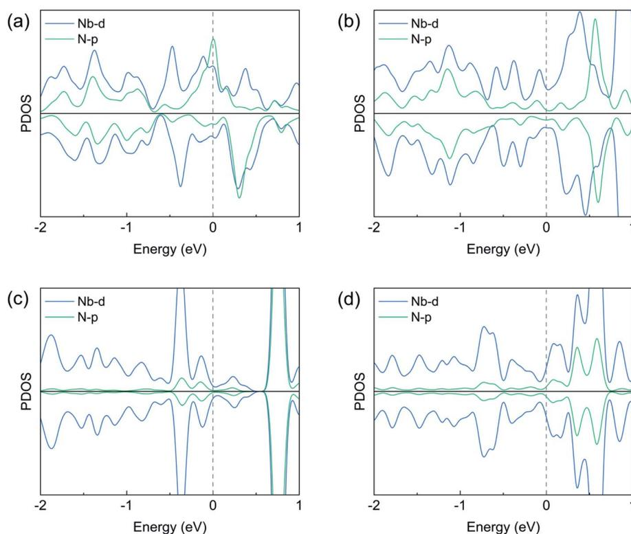
Fig. 4 Projected electronic density of states of  $N_2$  adsorbed on (a) zigzag edge and (b) zigzag edge with one Se vacancy *via* side-on pattern, (c) armchair edge and (d) armchair edge of  $NbSe_2$  *via* end-on pattern, respectively.
