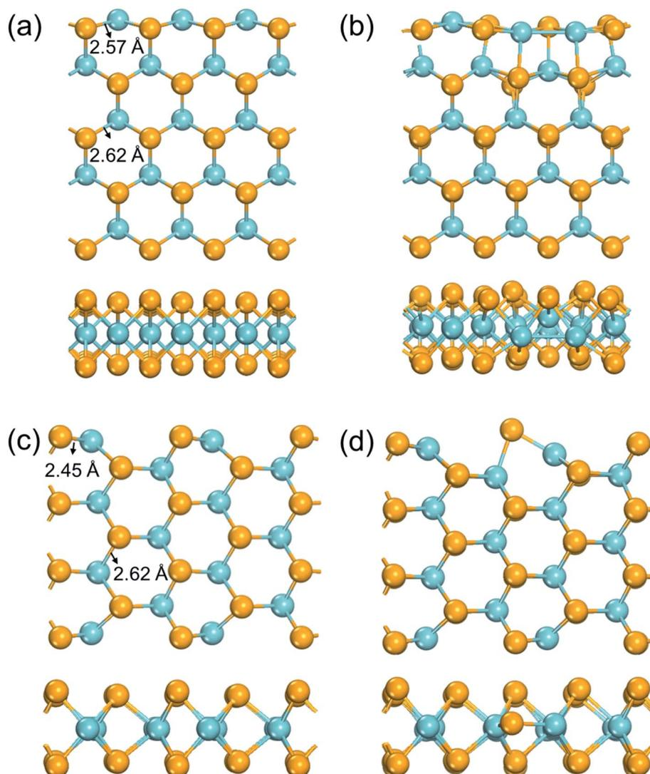
Fig. 1 Schematic view of the structure of the edges. (a) Pristine zigzag edge; (b) zigzag edge with a Se vacancy; (c) pristine armchair edge; (d) armchair edge with a Se vacancy. Mustard and teal balls represent Se and Nb atoms, respectively.
