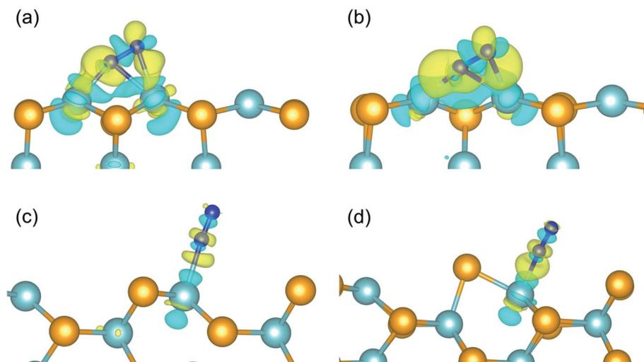
Fig. 3 The difference charge density of  $N_2$  adsorbed on (a) pristine zigzag edge, (b) zigzag edge with a Se vacancy, (c) pristine armchair edge, and (d) armchair edge with a Se vacancy. The isosurface value is set to be  $0.005 e \text{ \AA}^{-3}$ . Positive (accumulation) and negative (depletion) variations in the charge density are depicted as yellow and cyan surfaces, respectively.
