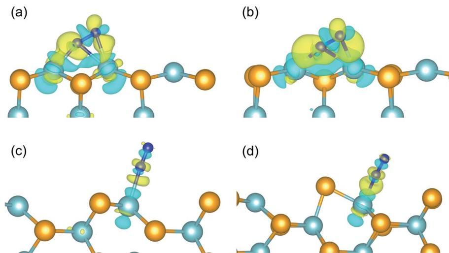
Fig. 3 The difference charge density of  $N_2$  adsorbed on (a) pristine zigzag edge, (b) zigzag edge with a Se vacancy, (c) pristine armchair edge, and (d) armchair edge with a Se vacancy. The isosurface value is set to be  $0.005 e \text{ \AA}^{-3}$ . Positive (accumulation) and negative (depletion) variations in the charge density are depicted as yellow and cyan surfaces, respectively.
