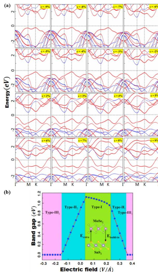
Fig. 9 (a) Under pressure, the band structures of MoSe<sub>2</sub>/SnS<sub>2</sub> heterojunctions. MoSe<sub>2</sub> and SnS<sub>2</sub> are represented by the red and blue lines, respectively. (b) The bandgap of MoSe<sub>2</sub>/SnS<sub>2</sub> heterojunctions varies as the external E-field changes. Reprinted from ref. 20 with permission from Elsevier, copyright 2021.
