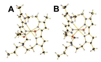
Fig. 2 Ball and stick representation of  $[ML(CH_3OH)(H_2O)](ClO_4)_2$  with M=Ni (A, 2) and M=Co (B, 3). Colour code: C, black; N, nitrogen; red, oxygen; light grey, hydrogen; green, nickel; pink, cobalt. Cocrystallised solvent molecules and counterions have been omitted for clarity.
