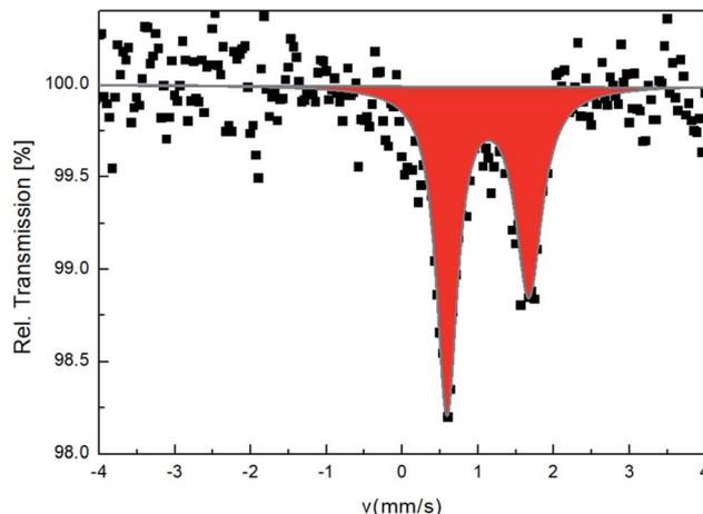
Fig. 4 <sup>57</sup>Fe Mössbauer spectrum of **4** at 293 K recorded in transmission geometry.
