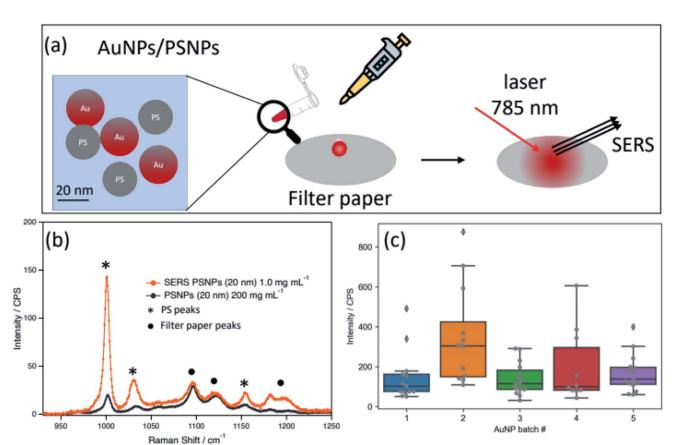
Fig. 1 (a) Schematic illustration for the filter paper system developed in this work, (b) representative surface-enhanced Raman spectra for PS(+)  $20 (1.0 \text{ mg mL}^{-1})$  with AuNP2 and unenhanced for PS(+) $20 (200 \text{ mg mL}^{-1})$ , and (c) box plots of surface-enhanced Raman intensities at  $1004 \text{ cm}^{-1}$  from each AuNP batch.
