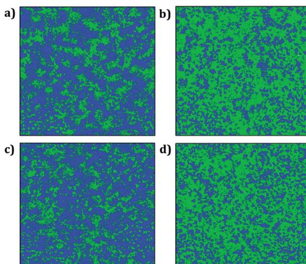
Fig. 8 Trajectory plots of Li and Na in (a)  $\text{Li}_2\text{NaOCl}$ , (b)  $\text{Na}_2\text{LiOCl}$ , (c)  $\text{Li}_2\text{NaOBr}$  and (d)  $\text{Na}_2\text{LiOBr}$  compounds after 2 ns. Blue and green lines represent the Li and Na trajectory lines, respectively.
