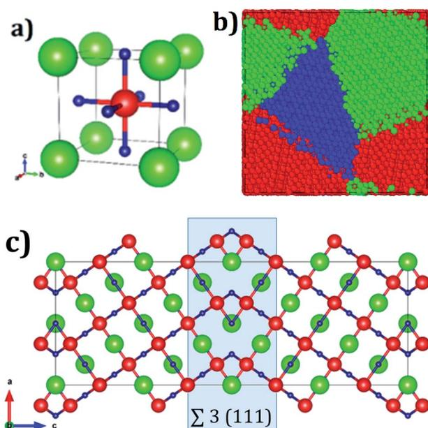
Fig. 1 (a) Unit cell of  $A_3OX$  ( $A = Li^+, Na^+$ ,  $X = Cl^-, Br^-$ ) lattice structures, green, red and blue represents  $X^-$ ,  $O^{2-}$  and  $A^+$  ions respectively, (b)  $A_3OX$  nanocrystal with three grains, and (c)  $\Sigma 3(111)$  grain boundary, where the shaded square highlights the grain boundary region. Color coding in (b) represents a unique grain.
