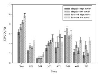
Fig. 5 CO/CO<sub>2</sub> ratio of the improved stove in comparison to the baseline stove with briquettes and raw coal during high power and low
