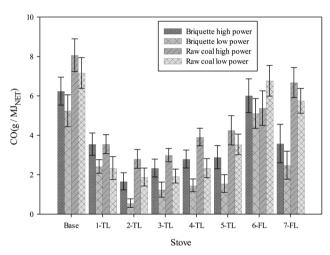
Fig. 6 Emission factors of CO from the improved stoves using briquettes and raw coal in comparison to the baseline stove.
