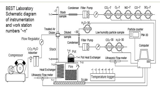
Fig. 1 Schematic diagram of the online testing system with work station  $\sim$ numbers (the H<sub>2</sub>O is a RH sensor. The  $\sim$ 30 and  $\sim$ 7 etc. are work stations numbers as indicated on the drawing).
