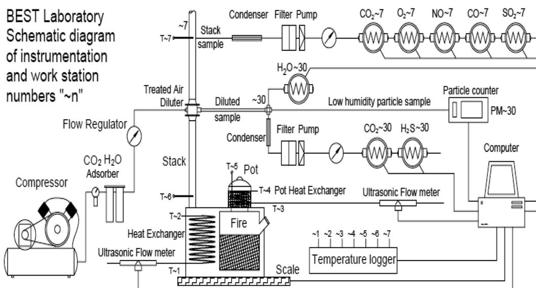
Fig. 1 Schematic diagram of the online testing system with work station ~numbers (the H<sub>2</sub>O is a RH sensor. The ~30 and ~7 etc. are work stations numbers as indicated on the drawing).
