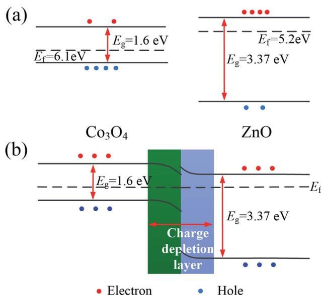
Fig. 9 Band structures of (a)  $\text{Co}_3\text{O}_4$  and ZnO and (b)  $\text{Co}_3\text{O}_4\text{-ZnO}$  heterojunction.
