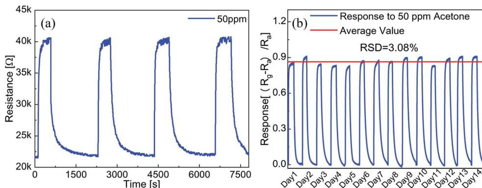
Fig. 5 (a) Cycle tests curves to 50 ppm acetone for  $\text{Pr}_{10}\text{Zn}_{40}\text{Co}_{50}$ . (b) Responses to 50 ppm acetone over two weeks.
