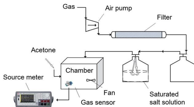
Fig. 1 Schematic diagram of gas sensing test system.
