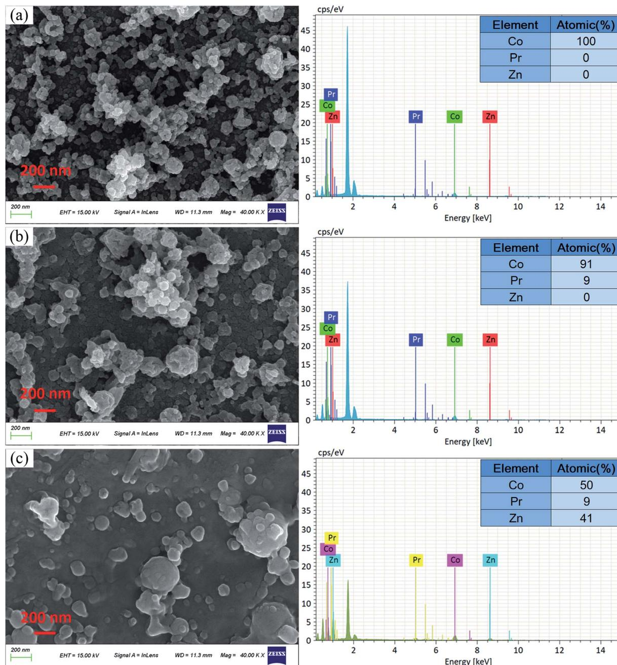
Fig. 6 SEM images and EDS spectra of (a) Co<sub>100</sub>, (b) Pr<sub>10</sub>Co<sub>90</sub> and (c) Pr<sub>10</sub>Zn<sub>40</sub>Co<sub>50</sub>.
