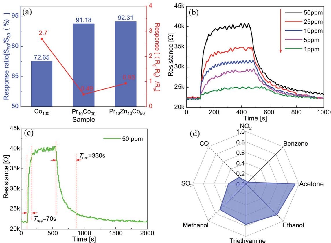
Fig. 4 (a) Responses to 50 ppm acetone and ratios of response at 90% and 30% relative humidity for  $\text{Co}_{100}$ ,  $\text{Pr}_{10}\text{Co}_{90}$  and  $\text{Pr}_{10}\text{Zn}_{40}\text{Co}_{50}$ . (b) Response–recovery curves to different concentrations of acetone. (c) Response–recovery curves to 50 ppm acetone. (d) Response to 50 ppm acetone and other gases.
