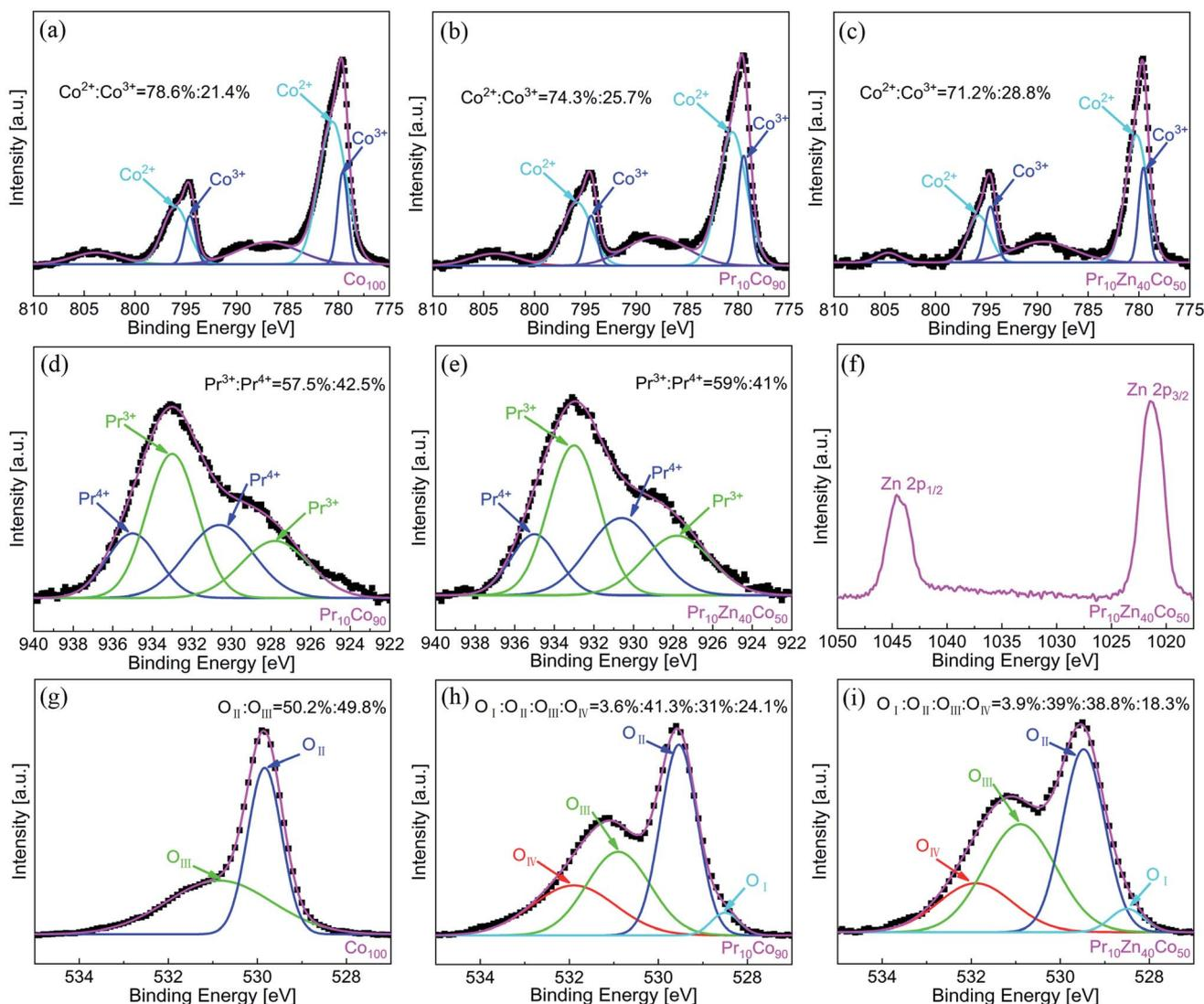
Fig. 8 High-resolution XPS spectra of (a and g)  $\text{Co}_{100}$ , (b, d and h)  $\text{Pr}_{10}\text{Co}_{90}$  and (c, e, f and i)  $\text{Pr}_{10}\text{Zn}_{40}\text{Co}_{50}$ .
