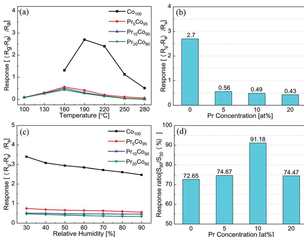
Fig. 2 Responses to 50 ppm acetone at (a) different temperature and (b) the optimal working temperature for  $\text{Co}_{100}$ ,  $\text{Pr}_5\text{Co}_{95}$ ,  $\text{Pr}_{10}\text{Co}_{90}$  and  $\text{Pr}_{20}\text{Co}_{80}$ . (c) Responses to 50 ppm acetone in different relative humidity, and (d) ratios of responses at 90% and 30% relative humidity for  $\text{Co}_{100}$ ,  $\text{Pr}_5\text{Co}_{95}$ ,  $\text{Pr}_{10}\text{Co}_{90}$  and  $\text{Pr}_{20}\text{Co}_{80}$ .
