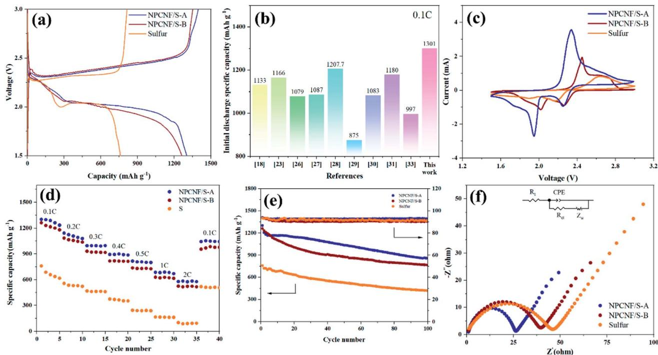
**Fig. 8** (a) The charge/discharge curves of sulfur, NPCNF/S-A, and NPCNF/S-B at 0.1C. (b) A comparison with initial discharge specific capacity at 0.1C. (c) The CV curves of sulfur, NPCNF/S-A, and NPCNF/S-B at 0.2 mV s<sup>-1</sup>. (d) The rate performances of sulfur, NPCNF/S-A, and NPCNF/S-B. (e) The cycling capacities and coulomb efficiency of sulfur, NPCNF/S-A, and NPCNF/S-B at 0.2C over 100 cycles. (f) EIS spectra and corresponding equivalent circuits of sulfur, NPCNF/S-A, and NPCNF/S-B.
