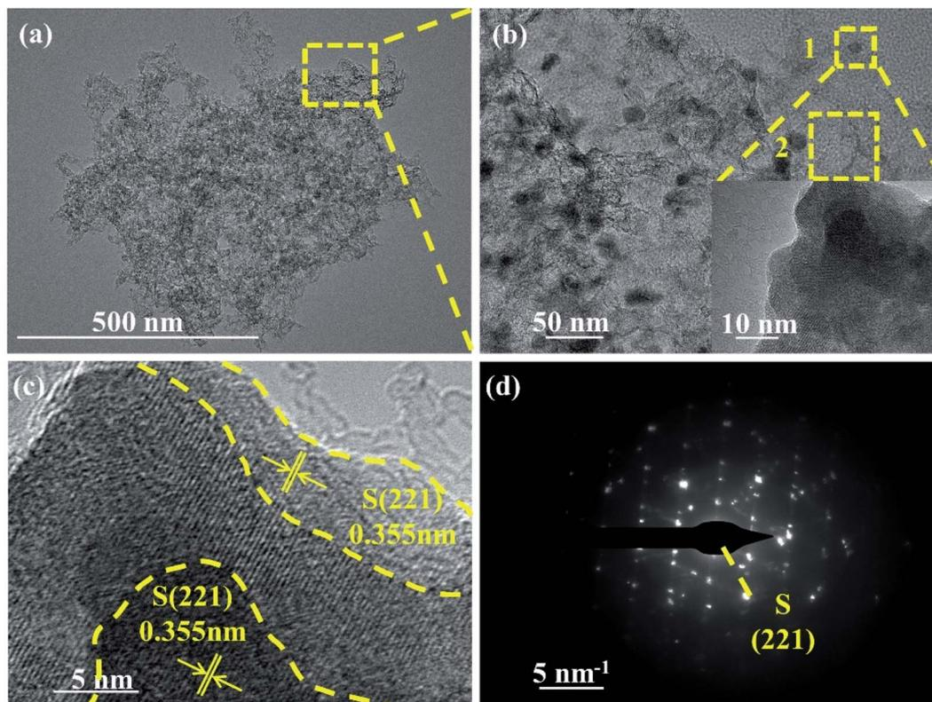
Fig. 5 (a) Low and (b) high-TEM images of NPCNF/S-A. (c) HRTEM images of area 1 in (b). (d) The SAED pattern of area 1 in (b).
