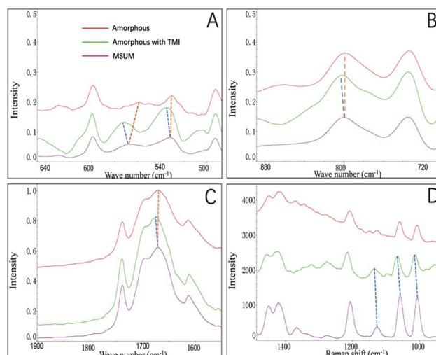
**Fig. 4** FTIR spectra details of amorphous form of MSUM in the absence/presence of TMI. (a) The oxygen–sodium peaks, (b) the –NH– peaks, (c) the –OH peaks of water molecules, and (d) Raman spectra details of amorphous form of MSUM in the absence/presence of TMI.
