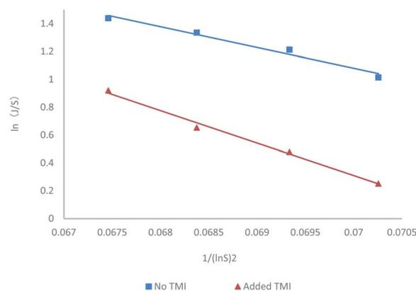
Fig. 2 Nucleation kinetics as a function of concentration ratio ( $S$ ), as predicted by the classical nucleation correlation, including 95% confidence intervals from linear regression. Nucleation rates are consistently slower upon the addition of a small amount of TMI.
