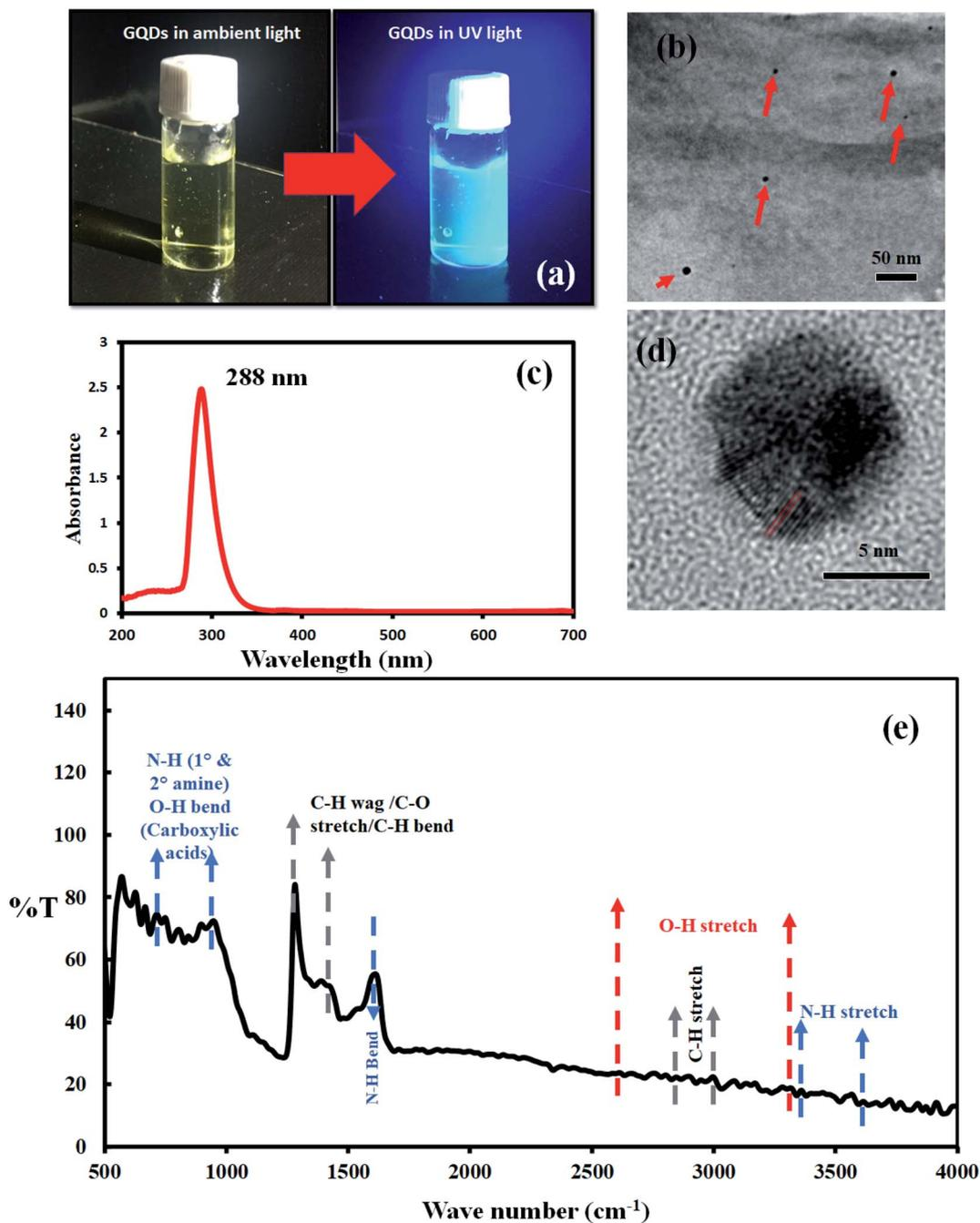
Fig. 2 (a) Visual observation of C-dots in ambient light and UV light (b) TEM image of C-dots (red arrow pointing C-dots) (c) UV-Vis spectrum (d) HRTEM image of a single C-dot with inter lattice spacing (0.24 nm) marked in red lines (e) FTIR of C-dots.
