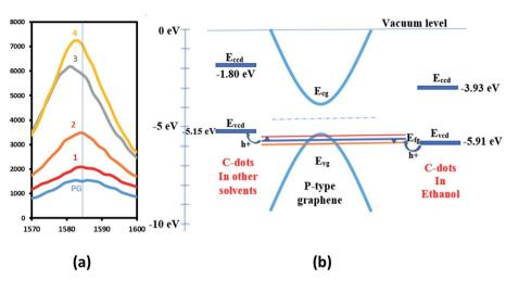
Fig. 4 (a) Shift in G band of graphene after C-dot doping (b) band diagram
