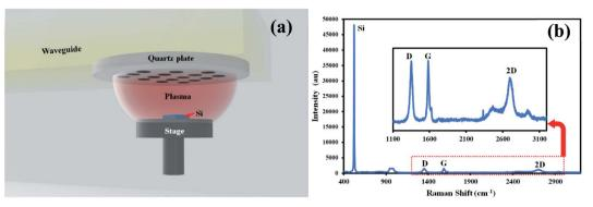
Fig. 1 Schematic diagram of microwave plasma CVD and Raman spectrum of the corresponding graphene
