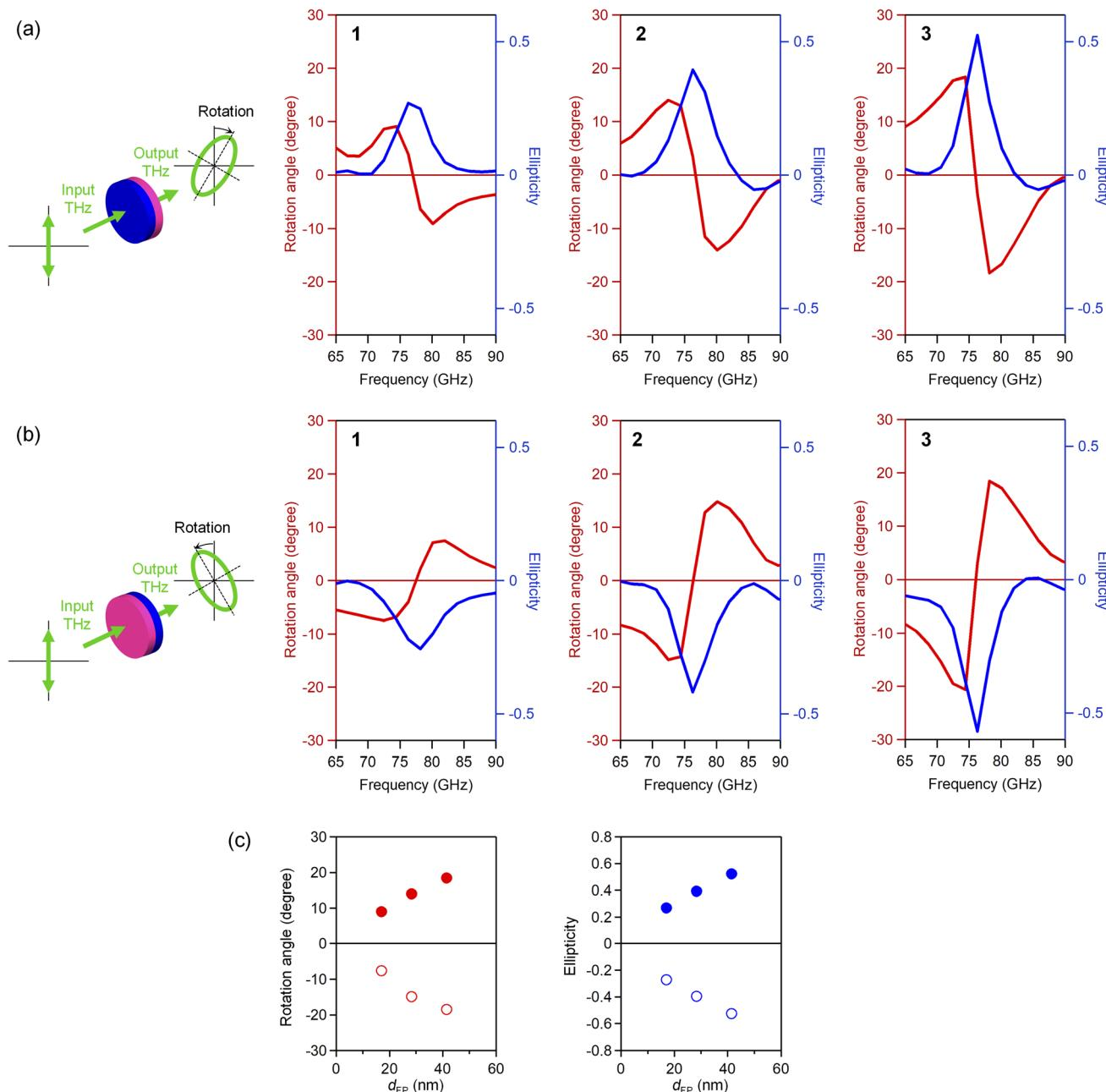
**Fig. 3** (a) and (b) Faraday rotation angle (red) and Faraday ellipticity (blue) measured by THz-TDS. The incident THz pulse was irradiated from S-pole (a) and N-pole (b) of the magnetized pellet sample. Left figures show the schematic illustration of the millimeter wave rotation. (c) Faraday rotation angle and Faraday ellipticity versus the particle size, measured by irradiating THz pulse from the S-pole side (close circles) and the N-pole side (open circles) of the magnetized pellets.
