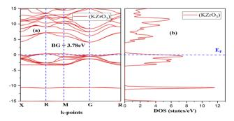
Fig. 3 (a) Band structure and (b) density of states (DOS) of the compound  $\mbox{KZrO}_3$ .
