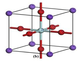
Fig. 1 Crystal structures of the compounds (a) RbZrO<sub>3</sub> and (b) KZrO<sub>3</sub>.
