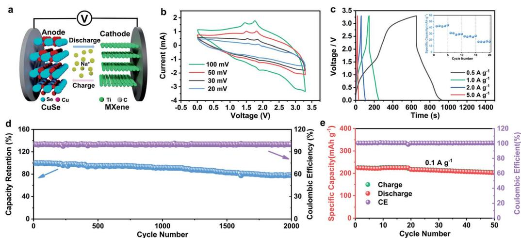
**Fig. 6** (a) Schematic of the CuSe// $\text{Ti}_3\text{C}_2\text{T}_x$  MXene SHIC device, (b) CV profiles at different scan rates, (c) GCD profiles of CuSe// $\text{Ti}_3\text{C}_2\text{T}_x$  MXene SHIC at various currents, (d) cycling performance of the CuSe// $\text{Ti}_3\text{C}_2\text{T}_x$  MXene SHIC at  $2 \text{ A g}^{-1}$ , and (e) cycling performance of the  $\text{Ti}_3\text{C}_2\text{T}_x$  MXene for SIBs.
