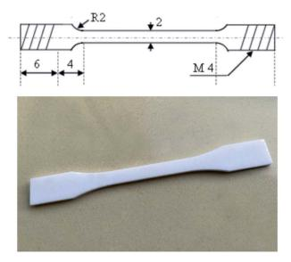
Fig. 12 Barbell type test strip.
