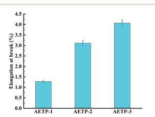
Fig. 15 Elongation at the break for different formulations.
