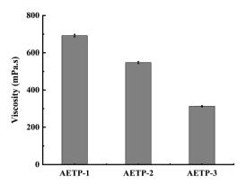
Fig. 11 Viscosity of different formulations at 0.1 s<sup>-1</sup> shear rate.
