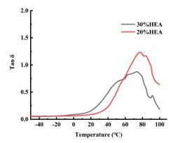
Fig. 6 DMA analysis of composite materials.
