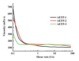
Fig. 10 Flow viscosity-shear rate curves of different formulations.
