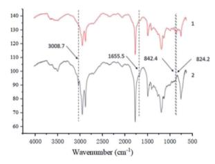
Fig. 3 Infrared spectra before and after tung oil epoxidation.
