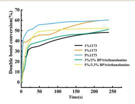
Fig. 7 Effect of initiators on the time-conversion rate.
