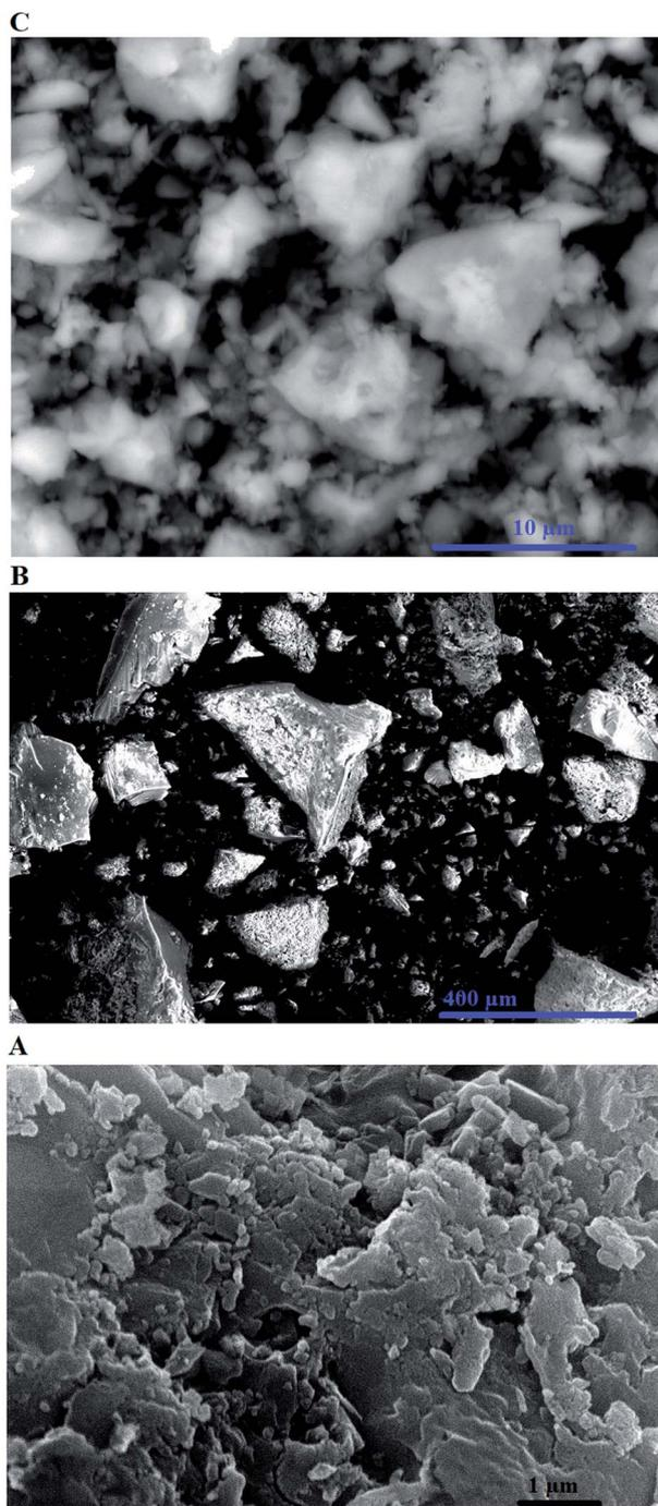
Fig. 4 The FE-SEM images of the SiO<sub>2</sub> (A), N<sub>1</sub> (B), and N<sub>2</sub> (C) samples.
