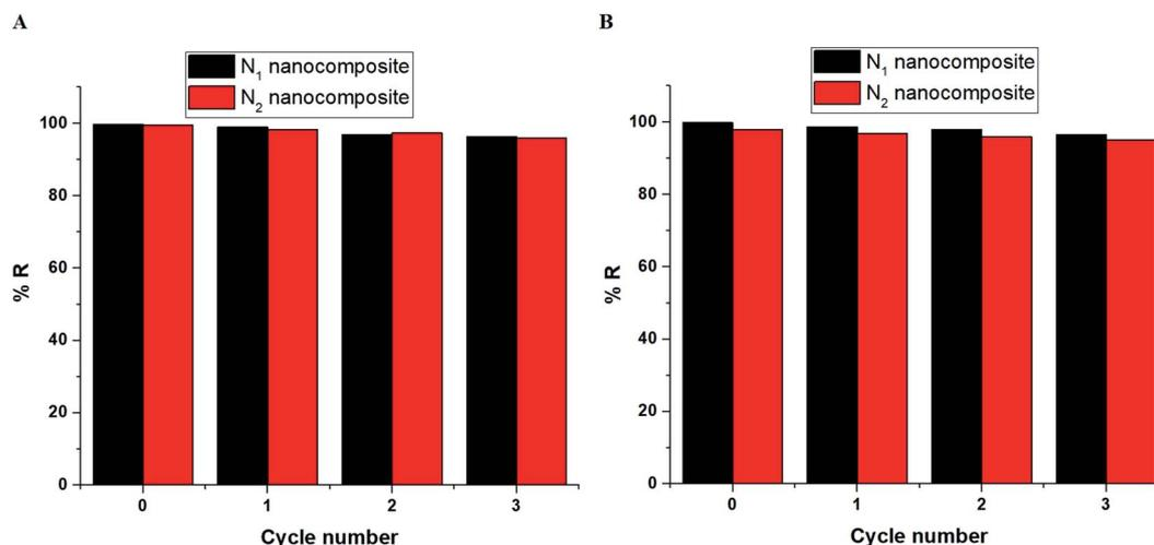
Fig. 15 The plot of % R or Q (mg g<sup>-1</sup>) versus cycle number in the case of Cu(II) (A) and Cd(II) (B) ions.
