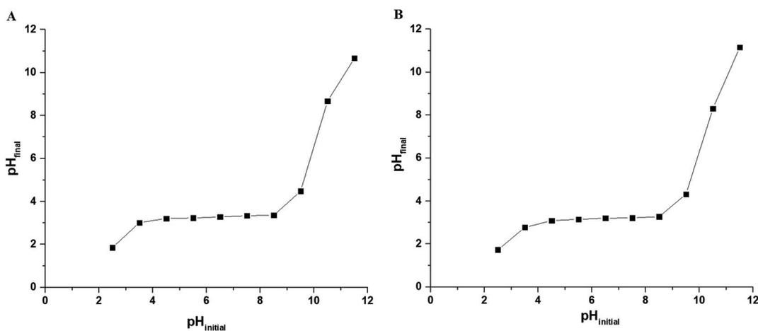
Fig. 6 The plot of pH<sub>final</sub> versus pH<sub>initial</sub> for several KCl solutions in the case of using N<sub>1</sub> (A) and N<sub>2</sub> (B) nanocomposites.
