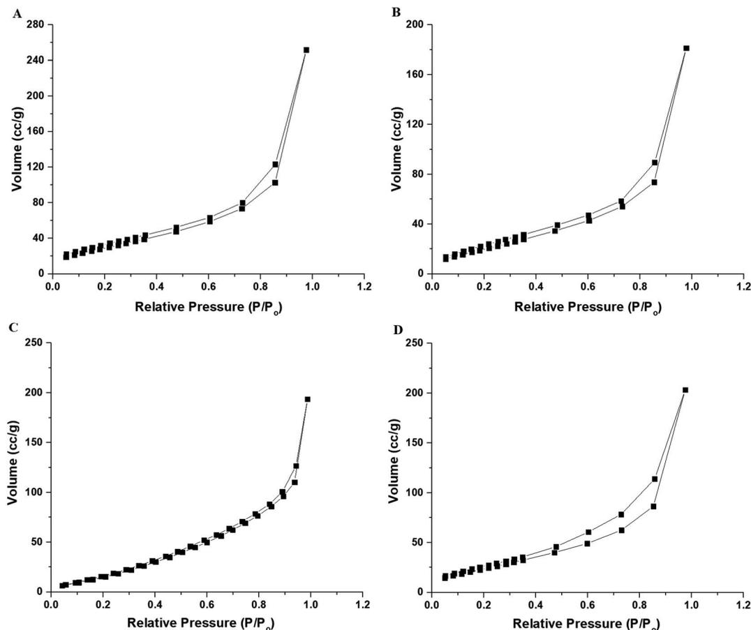
Fig. 3 The  $N_2$  adsorption/desorption isotherms of the  $SiO_2$  (A),  $SiO_2/(3\text{-aminopropyl})\text{triethoxysilane}$  (B),  $N_1$  (C), and  $N_2$  (D) samples.
