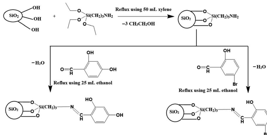
Scheme 1 The proposed structure of the synthesized nanocomposites.
