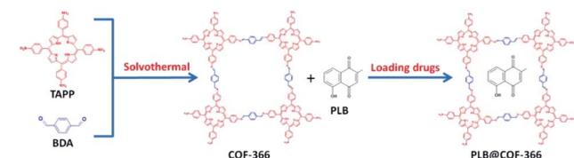
Fig. 1 Schematic illustration of the preparation process of nanoscale COF-366 and PLB@COF-366.
