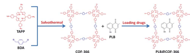
Fig. 1 Schematic illustration of the preparation process of nanoscale COF-366 and PLB@COF-366.
