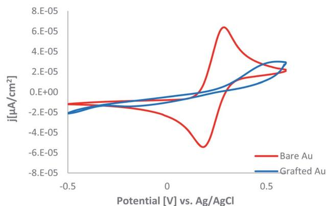
Fig. 2 Cyclic voltammograms recorded in aqueous solution of ferri-cyanide/ferricyanide ions (5.0 mM  $\text{Fe}(\text{CN})_6^{3-/4-}$  in 100 mM KCl) on bare and modified gold electrode (modification by cyclic voltammetry, at potential range from +0.2 V to +1.6 V).
