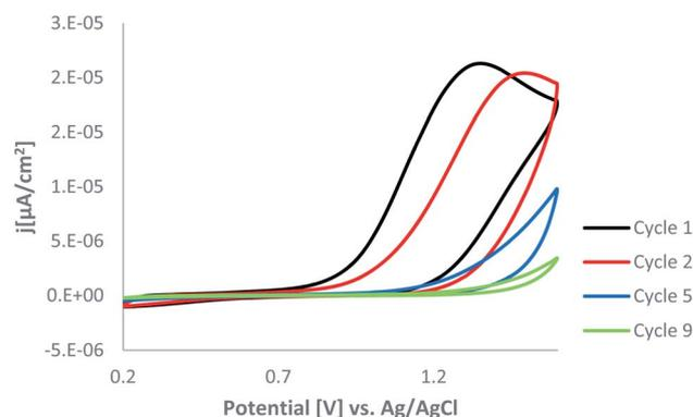
Fig. 1 Cyclic voltammograms recorded at the gold electrode with diameter  $d = 0.2$  cm immersed in 3-amino-1,2,4-triazole (2 mM) solution after addition of (50 mM) NBu<sub>4</sub>BF<sub>4</sub> to 20 ml acetonitrile. Scanning potential  $v = 100$  mV s<sup>–1</sup> and applied potential range from +0.2 to +1.6 V [black (first cycle), red (second cycle), blue (fifth cycle), green (ninth cycle)].
