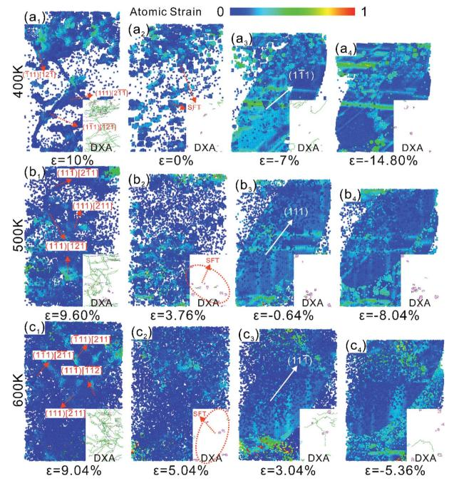
Fig. 6 The microstructural evolution of NSCA under tension-compression loading at temperatures from 400 K to 600 K. The simulated temperatures are 400 K for (a), 500 K for (b) and 600 K for (c), retaining atoms in the range 4 < CSP < 11 and performing dislocation analysis using DXA (staining of the atoms by shear strain).
