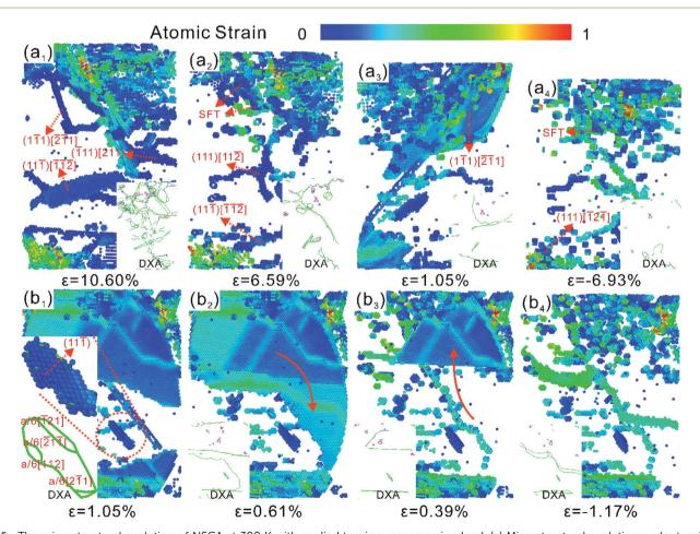
Fig. 5 The microstructural evolution of NSCA at 300 K with applied tension—compression load. (a) Microstructural evolution under tension—compression loading. (b) Appearance and disappearance of twins after compressive yielding. Atoms in the range 4 < CSP < 11 were retained and dislocation analysis was performed using DXA. The dashed arrows in the figure mark the dislocation lines and the solid arrows indicate the trend of twin movement.
