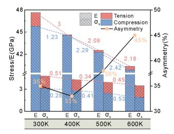
Fig. 2 Elastic modulus, yield stress and tensile-compression asymmetry coefficient of NSCA under tensile and compressive loads at 300-600 K. Values represent the magnitude of the difference between the adjacent tensile (red) and compressive (blue) yield stress and modulus of elasticity, with dashed lines linking the adjacent tensile (red) and compressive (blue) yield stress and modulus of elasticity.
