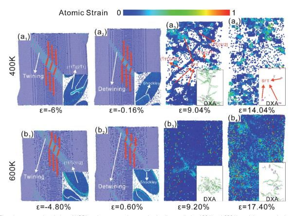
Fig. 9 The microstructural evolution of NSCA under compression—tension loading applied at 400 K and 600 K, retaining atoms in the range 4 < CSP < 11 and using DXA for dislocation analysis (staining of the atoms by shear strain). (a) 400 K, (b) 600 K.
