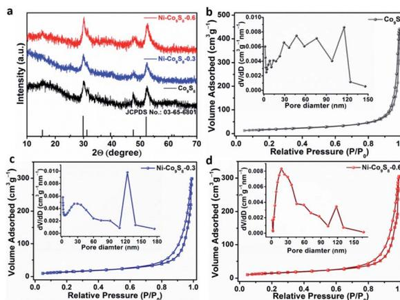
Fig. 3 (a) XRD patterns of  $Ni_xCo_{9-x}S_8$  series hollow spheres. Nitrogen adsorption–desorption isotherms and the corresponding pore size distributions (inset) of (b)  $Co_9S_8$ , (c)  $Ni-Co_9S_8-0.3$ , and (d)  $Ni-Co_9S_8-0.6$  hollow spheres.
