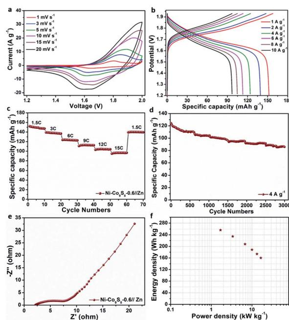
Fig. 6 The electrochemical characterization of  $\text{Ni-Co}_9\text{S}_8-0.6//\text{Zn}$  battery (a) CV curves, (b) GCD curves, (c) rate capability, (d) the cyclic stability at  $4 \text{ A g}^{-1}$ , (e) Nyquist plot, and (f) Ragone plot.
