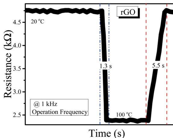
Fig. 5 Response and recovery time for the rGO-based temperature sensor.
