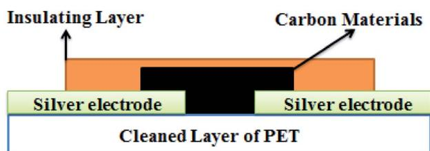
Fig. 1 Schematic diagram of a flexible temperature sensor.
