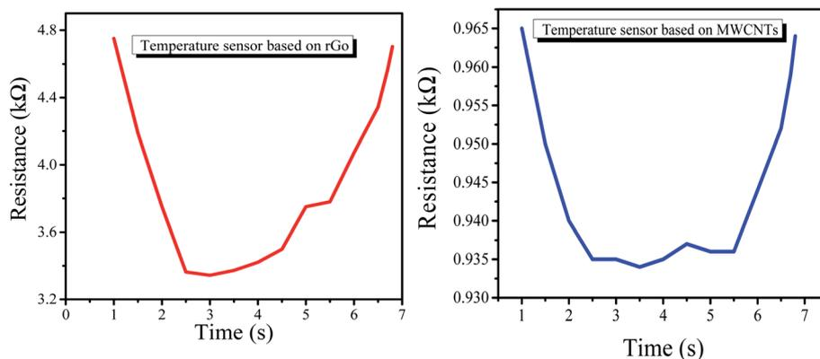
Fig. 7 Resistance output of the temperature sensors.
