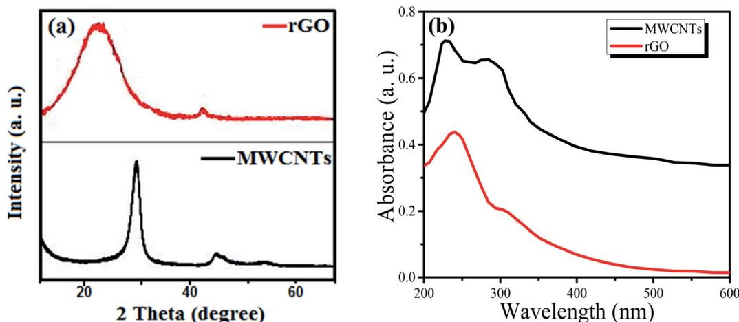
Fig. 3 (a) XRD patterns of reduced graphene and multi-walled carbon nanotubes. (b) UV-Vis absorbance of reduced graphene and multi-walled carbon nanotubes.
