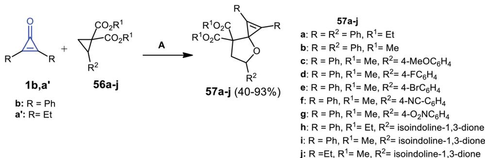
Scheme 37 Sc(OTf)<sub>3</sub> mediated the synthesis of **57a-j**. Reagents and conditions: A = Sc(OTf)<sub>3</sub> (10 mol%), DCM, 25 °C 4 h.
