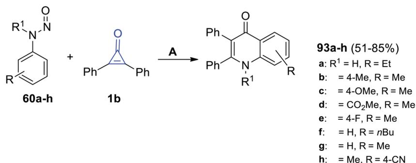
**Scheme 59** Synthesis of 4-quinolones **93a-h**. Reagents and conditions: A = [RhCp\*(OAc)<sub>2</sub>] (0.5 mol%), [Rh(COD)Cl]<sub>2</sub>, AgBF<sub>4</sub> (0.02 mmol), DCM, 120 °C, 36 h.
