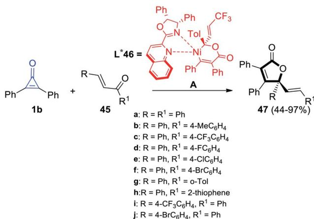
Scheme 31 Synthesis of  $\gamma$ -alkenylbutenolide **47** from enones **45** and **1b**. Reagents and conditions: A = Ni(cod)<sub>2</sub> (1–2 mol%), L\* **46** (2–3 mol%), toluene, rt, 1–24 h.
