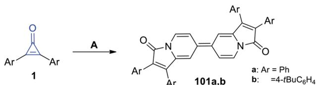
Scheme 63 Synthesis of biindolizines **101a,b**. Reagents and conditions: A = pyridine, Cu(OAc)<sub>2</sub>, 15 min.
