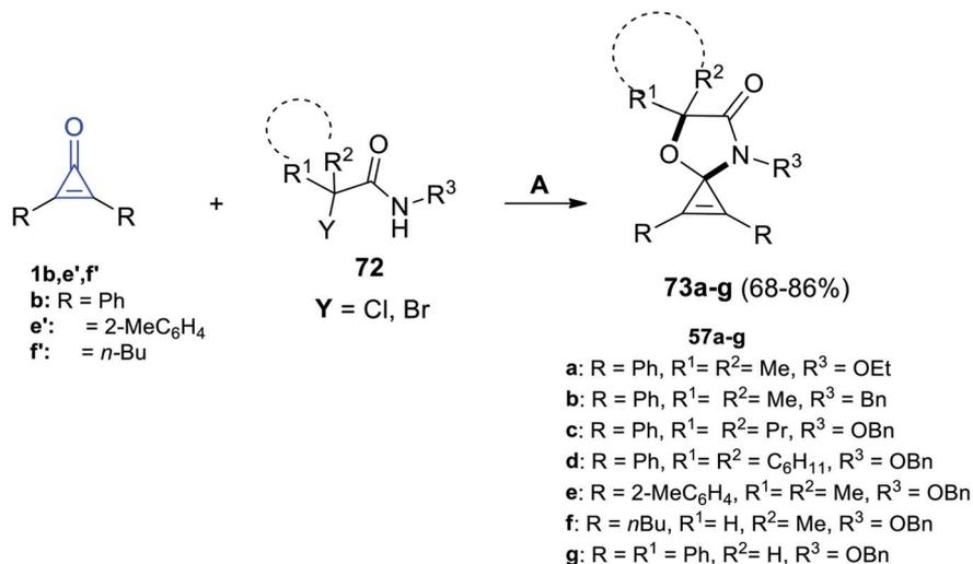
Scheme 43 Synthesis of spiro oxazoles **73a–g**. Reagents and conditions: A = K<sub>2</sub>CO<sub>3</sub> (0.8 mmol), HFIP (2 ml), 50 °C, 12 h.
