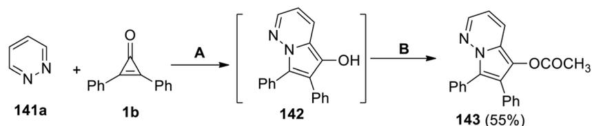
Scheme 87 Synthesis of 6,7-diphenylpyrrolo[1,2-*b*]pyridazin-5-yl acetate (**143**). Reagents and conditions: A = DCE, reflux, B = Ac<sub>2</sub>O, DMAP.
