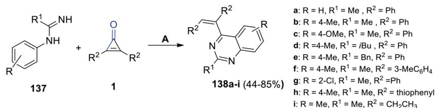
Scheme 85 Synthesis of quinazoline derivatives **138a-i**. Reagents and conditions: A = (Cp\*RhCl<sub>2</sub>)<sub>2</sub>, AgSbF<sub>6</sub>, DCM, reflux, 36 h, O<sub>2</sub>.
