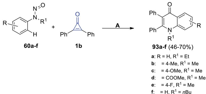
**Scheme 58** Rhodium(III)-catalyzed synthesis of quinoline-4-one derivatives **93a-f**. Reagents and conditions: A = (Cp\*RhCl<sub>2</sub>)<sub>2</sub> (2 mol%), AgBF<sub>4</sub> (1.2 equiv.), NaF, DCE, 100 °C, 12 h.
