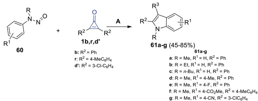
Scheme 39 Synthesis of indoles **61a–g**. Reagents and conditions: A = [RhCp\*(OAc)<sub>2</sub>], AgNTf<sub>2</sub>, DCE, 120 °C, 24 h.
