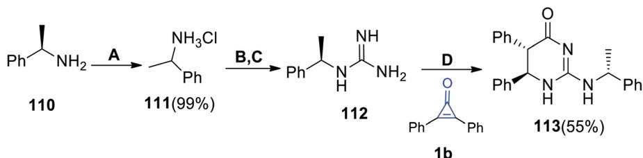
Scheme 68 Synthesis of 5,6-dihydropyrimidine **113**. Reagents and conditions: A = conc. HCl, 1,4 dioxane, 20 °C; B =  $\text{NH}_2\text{CN}$ , pH 8–9,  $\text{H}_2\text{O}$ , reflux, 5 h; C = passed through Amberlite IRA-401 (hydroxide form); D = benzene : EtOH (1 : 1), rt, 18 h.
