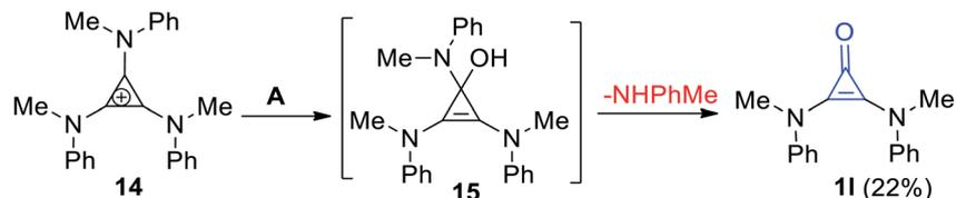
Scheme 11 Formation of 2,3-bis(methyl(phenyl)-amino)cycloprop-2-enone (**11**). Reagents and conditions: A = KOH/H<sub>2</sub>O, MeOH, rt, 40 h.
