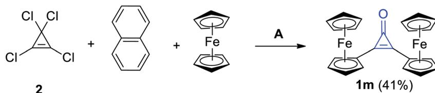
Scheme 12 Synthesis of diferoencylcyclopropenone (**1m**). Reagents and conditions: A = AlCl<sub>3</sub>, CH<sub>2</sub>Cl<sub>2</sub>, H<sub>2</sub>O.
