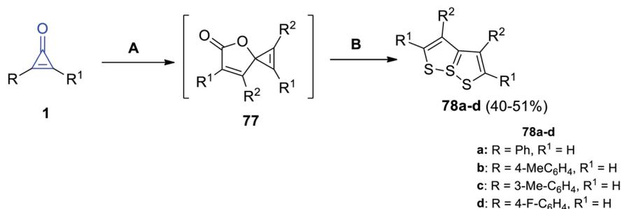
Scheme 47 Synthesis of [1,2]dithiolo[5,1-e][1,2]dithioles **78a–d**. Reagents and conditions: A = CuBr (5 mol%), DCM, 75 °C, N<sub>2</sub>, 12 h, B = KF (2 equiv.), S<sub>8</sub>, DMF, 50 °C, air, 5 h.
