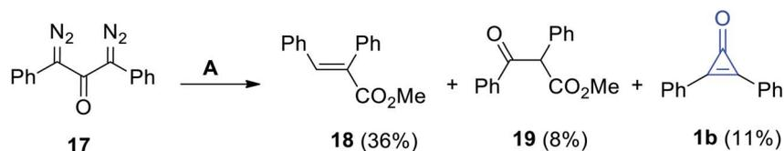
Scheme 14 Oxidation of **17** into diphenylcyclopropenone (**1b**), **18** and **19**. Reagents and conditions: A = MeOH, Ag<sub>2</sub>O.
