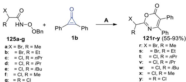
Scheme 78 Synthesis of substituted 1,3-oxazin-6-ones **123r-y**. Reagents and conditions: A = DCM, reflux, Et<sub>3</sub>N, 2 h.
