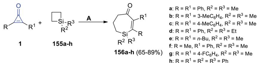
Scheme 92 Synthesis of tetrasubstituted-6,7-dihydro-1*H*-silepin-4(5*H*)-ones **156a–h**. Reagents and conditions: A = (1 mol%), Pd(OAc)<sub>2</sub> toluene, rt, 48 h.
