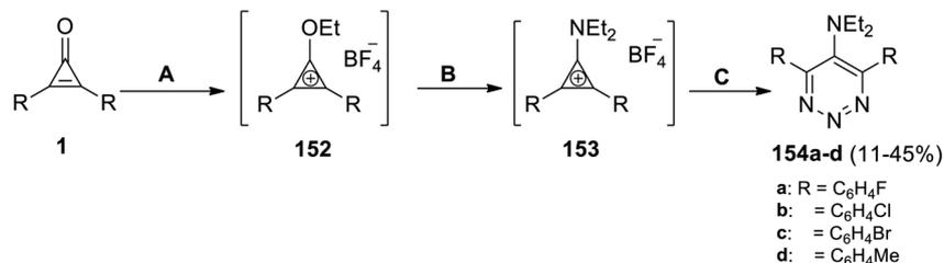
Scheme 91 Synthesis of triazines (**154a–d**). Reagents and conditions: A = Et<sub>3</sub>OBF<sub>4</sub>, CH<sub>2</sub>Cl<sub>2</sub>; B = Et<sub>2</sub>NH; C = NaN<sub>3</sub>, CH<sub>2</sub>Cl<sub>2</sub>, DMF.
