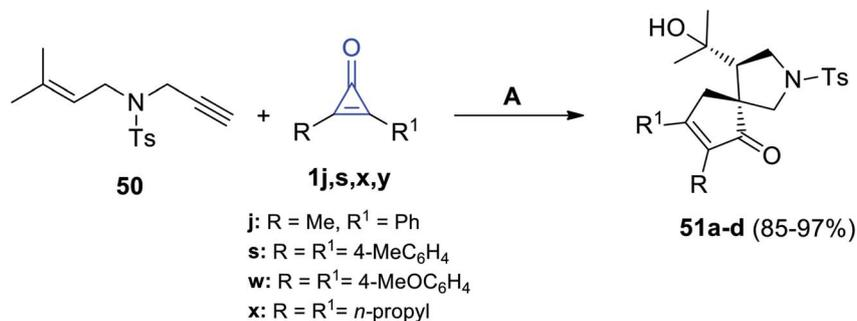
Scheme 34 (IPr)AuNTf<sub>2</sub>-catalyzed synthesis of compounds **51a–d**. Reagents and conditions: A = (IPr)AuNTf<sub>2</sub> (2 mol), DCM, rt.
