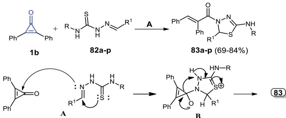
Scheme 50 Synthesis and mechanism of thiadiazoles **83a-p**. Reagents and conditions: A = EtOH, 4–8 h.Table 1 Substituents and the yield of thiadiazoles **83a-p**
