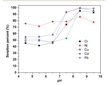
Fig. 6 Effect of pH on the sorption percentage. Utilized conditions:  $Cr^{3+}$ ,  $Ni^{2+}$ ,  $Cu^{2+}$ ,  $Cd^{2+}$ , and  $Pb^{2+}$  50  $\mu g$  L; volume: 50 mL; PAN: 2  $\times$  10<sup>-5</sup> mol.L<sup>-1</sup>; flow rate: 0.8 mL.min<sup>-1</sup>.
