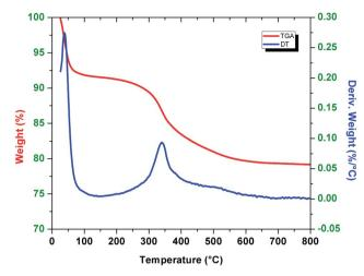
Fig. 2 Thermal gravimetric analysis diagram of SiO<sub>2</sub>-(CH<sub>2</sub>)<sub>3</sub>-Im-C<sub>18</sub>.
