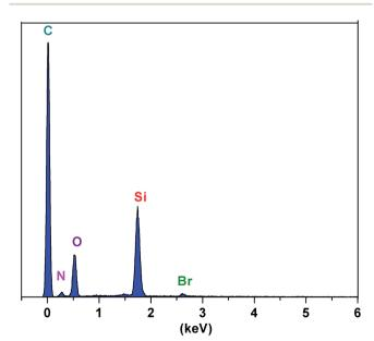
Fig. 3 Energy-dispersive X-ray spectroscopy of  $SiO_2$ -(CH<sub>2</sub>)<sub>3</sub>-Im-C<sub>18</sub>.
