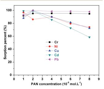
Fig. 7 Effect of PAN concentration on  $SiO_2-(CH_2)_3-Im-C_{18}$ . Utilized conditions:  $Cr^{3+}$ ,  $Ni^{2+}$ ,  $Cu^{2+}$ ,  $Cd^{2+}$ , and  $Pb^{2+}$  50  $\mu g$  L; volume: 50 mL; flow rate: 0.8 mL.min<sup>-1</sup>.
