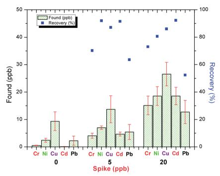
Fig. 11 Determination of  $Cr^{3+}$ ,  $Ni^{2+}$ ,  $Cu^{2+}$ ,  $Cu^{2+}$ , and  $Pb^{2+}$  in water samples. Average of three determinations  $\pm$  standard deviation (SD), n=3.
