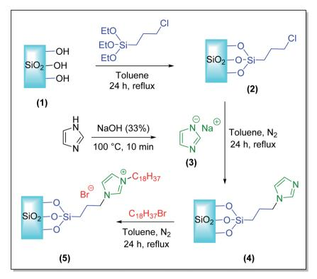
Scheme 1 Synthetic procedure of SiO<sub>2</sub>-(CH<sub>2</sub>)<sub>3</sub>-Im-C<sub>18</sub>
