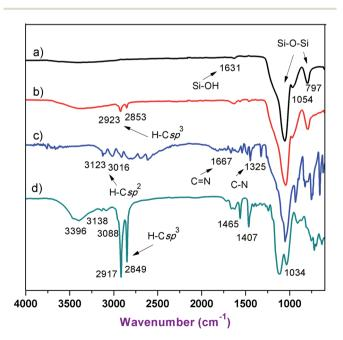
Fig. 1 FT-IR spectra of (a) SiO<sub>2</sub> (1), (b) SiO<sub>2</sub>-(CH<sub>2</sub>)<sub>3</sub>-Cl (2), (c) SiO<sub>2</sub>-(CH<sub>2</sub>)<sub>3</sub>-Im (4), (d) SiO<sub>2</sub>-(CH<sub>2</sub>)<sub>3</sub>-Im-C<sub>18</sub> (5).
