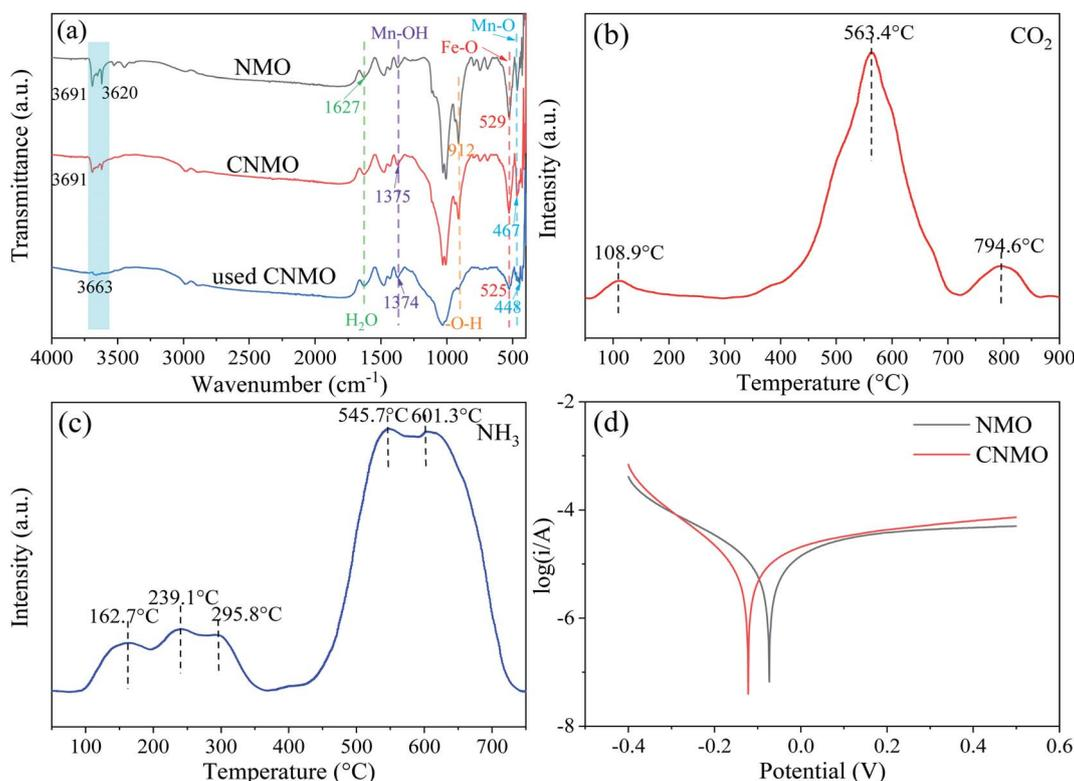
Fig. 3 (a) FTIR spectra of NMO, CNMO and used CNMO; (b) CO<sub>2</sub>-TPD, (c) NH<sub>3</sub>-TPD and (d) Tafel polarization profiles of CNMO.
