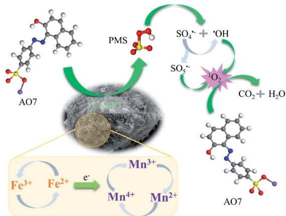
Scheme 1 Schematic illustration of PMS activation mechanism for AO7 degradation in CNMO/PMS system.
