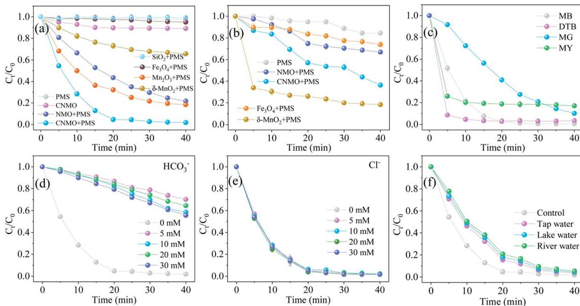
Fig. 5 Degradation of (a) AO7 and (b) PMS residues in various systems; (c) degradation of different pollutants in the CNMO/PMS system; the influence of (d) inorganic anions  $\text{HCO}_3^-$  and (e)  $\text{Cl}^-$  on the degradation of AO7 in the CNMO/PMS system; (f) AO7 removal in actual water (conditions:  $C_0 = 20 \text{ mg L}^{-1}$ ,  $M_{\text{CNMO}} = 0.9 \text{ g L}^{-1}$ ,  $M_{\text{PMS}} = 0.15 \text{ mM}$ ,  $\text{pH} = 6.6$ ,  $T = 25 \text{ }^\circ\text{C}$ ).
